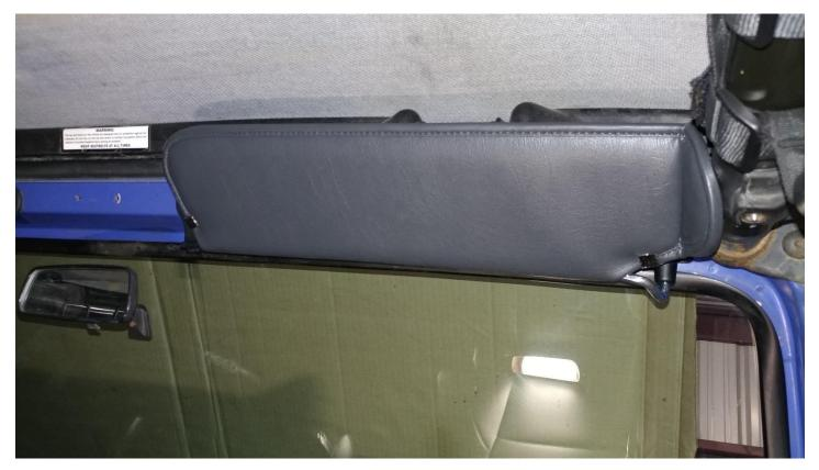
6. Remove the 2 – T20 Torx head screws from the diver side.
