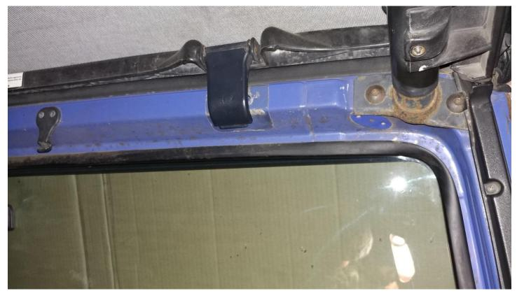
4. Line up the new sun visor with the existing factory holes. Reinstall the 2 – T20 Torx head screws
