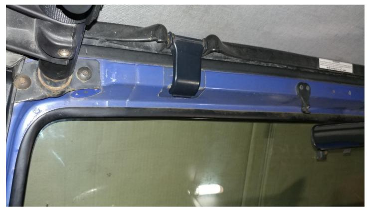
8. Line up the new sun visor with the existing factory holes. Reinstall the 2 – T20 Torx head screws
