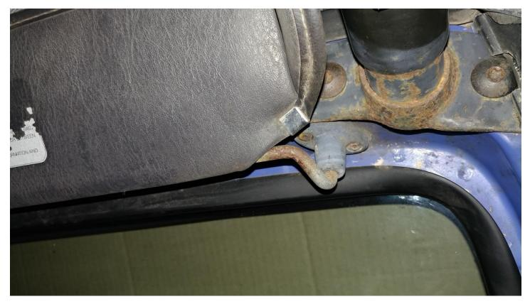
3. After removing the screws the old sun visor will be free.
