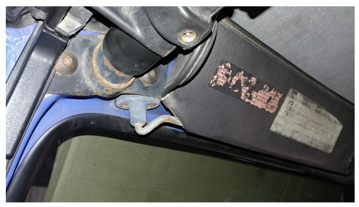
7. After removing the 2 screws the old sun visor will be free.
