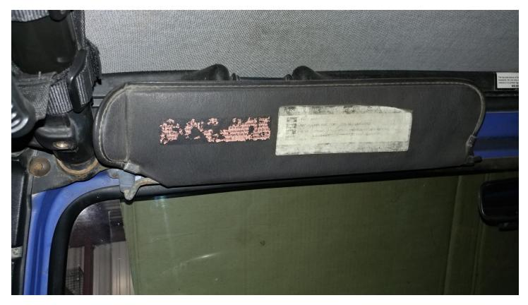
2. I started with the passenger side. Remove the 2 - T20 Torx head screws.
