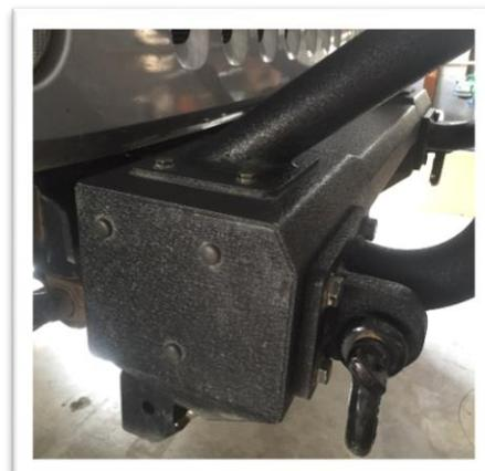
2. Remove the plastic plugs from the sides of the bumper if present.
