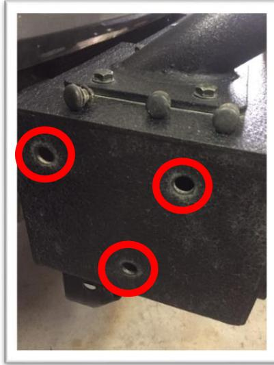
3. Attach stubby ends to the bumper using M12 hardware. Bolt heads should be inside stubby ends and lock nuts inside center section.
