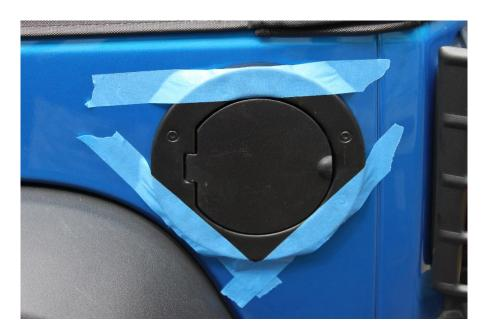
4. Open the door and locate the mounting tabs inside the cover. There are four (4). Two (2) upper and two (2) lower.
