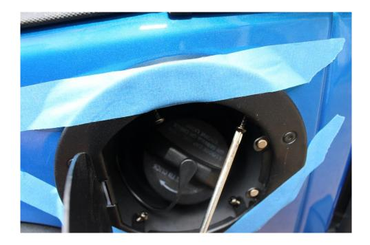
7. Working around tighten all the screws. You may use an electric screw driver or a drill but do not overtighten.
