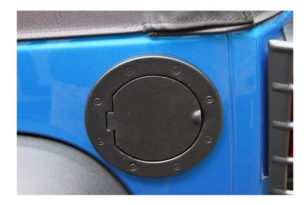
3. If you are working alone tape the door in place with masking tape so it does not move during installation.
