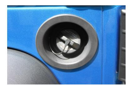
2. Place gas cap door over the plastic housing with the opening facing the rear of the Jeep as shown. Make sure the door is level. You can check this with a small level or eye ball it.
