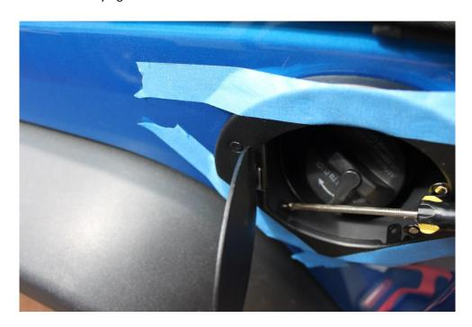
6. Working in a X pattern start all four screws.
