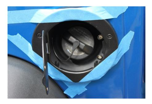
5. Starting on the bottom start the screws. Screws are self-tapping and will require some pressure but should not require a pilot hole. Do not fully tighten screws at this time.
