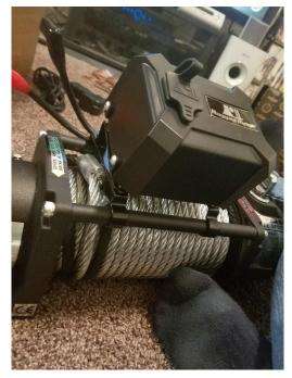
5. Attach the wires from the solenoid box to the winch using the picture below for reference and tighten the bolts using a 14 mm wrench. Pull the rubber caps over the bolts to help seal the connections. The small black wire goes to the bottom bolt of the motor side of the winch as well as the supplied long black cable.
