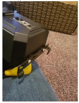
2. Solenoid Mounting Option 2 (Vertical Mount): Bolt together the 2 90 degree brackets and the 2 bar brackets using the provided allen bolts and nuts. Take the solenoid and mount the other side of the 90 degree brackets to the bottom of the solenoid. Place the assembly over the winch bars and using the provided allen bolts secure the assembly to the winch.
