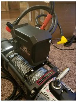
3. Solenoid Mounting Option 4 (Flat Mount): using only the two winch bar brackets mount the brackets to the bottom of the solenoid and then secure the brackets to the winch bars, all using the supplied allen bolts and nuts.
