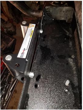
7. Slide the 4 square nuts into the slots on the feet of the winch (it may be helpful to secure these with tape in order for them to not fall out). Place the winch onto the bumper and using the 4 16 mm bolts and locking washers secure the winch to the bumper (it may be helpful now to unwrap some of the winch line and feed it through the fairlead).
