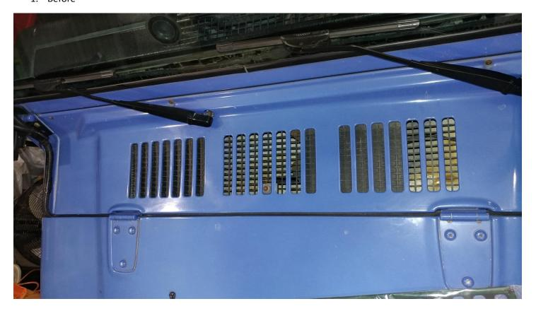
2. Remove the T15 screw from the center of the Hood Vent.
