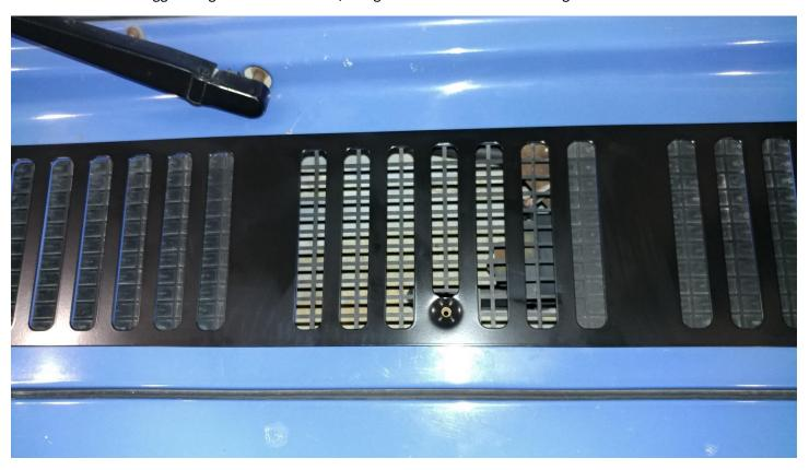
7. Apply pressure to the areas of contact and install the new provided Philips head screw
