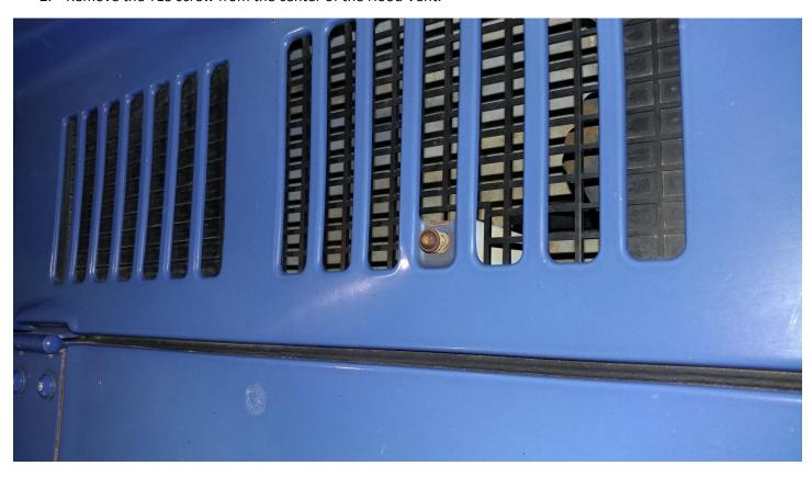
3. Line up the new Rugged Ridge Hood Vent Cover, so that you can see where the Jeep should be cleaned and how the cover will fit.
