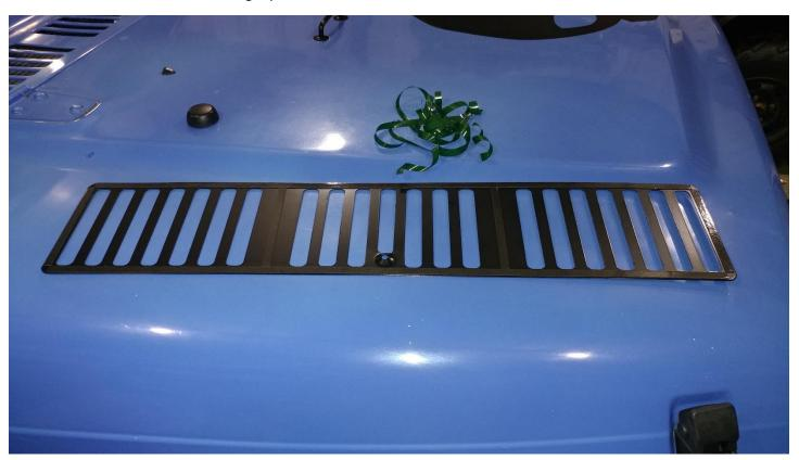
6. Locate the Rugged Ridge Hood Vent Cover, using the center screw hole to align it.
