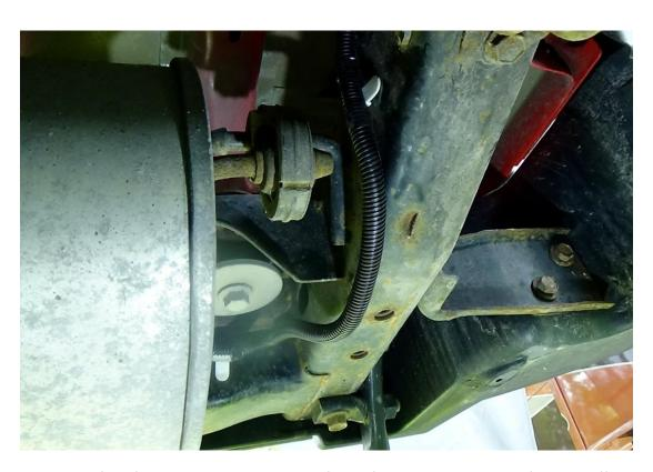
down the inside of the frame rail. Be sure it goes in front of and above the hanger for the muffler.
