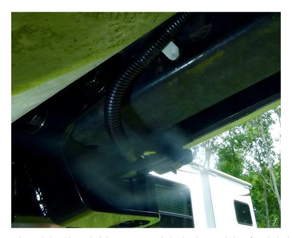
you go, then push the rubber trailer light connector into the bracket that extends down from the hitch.
