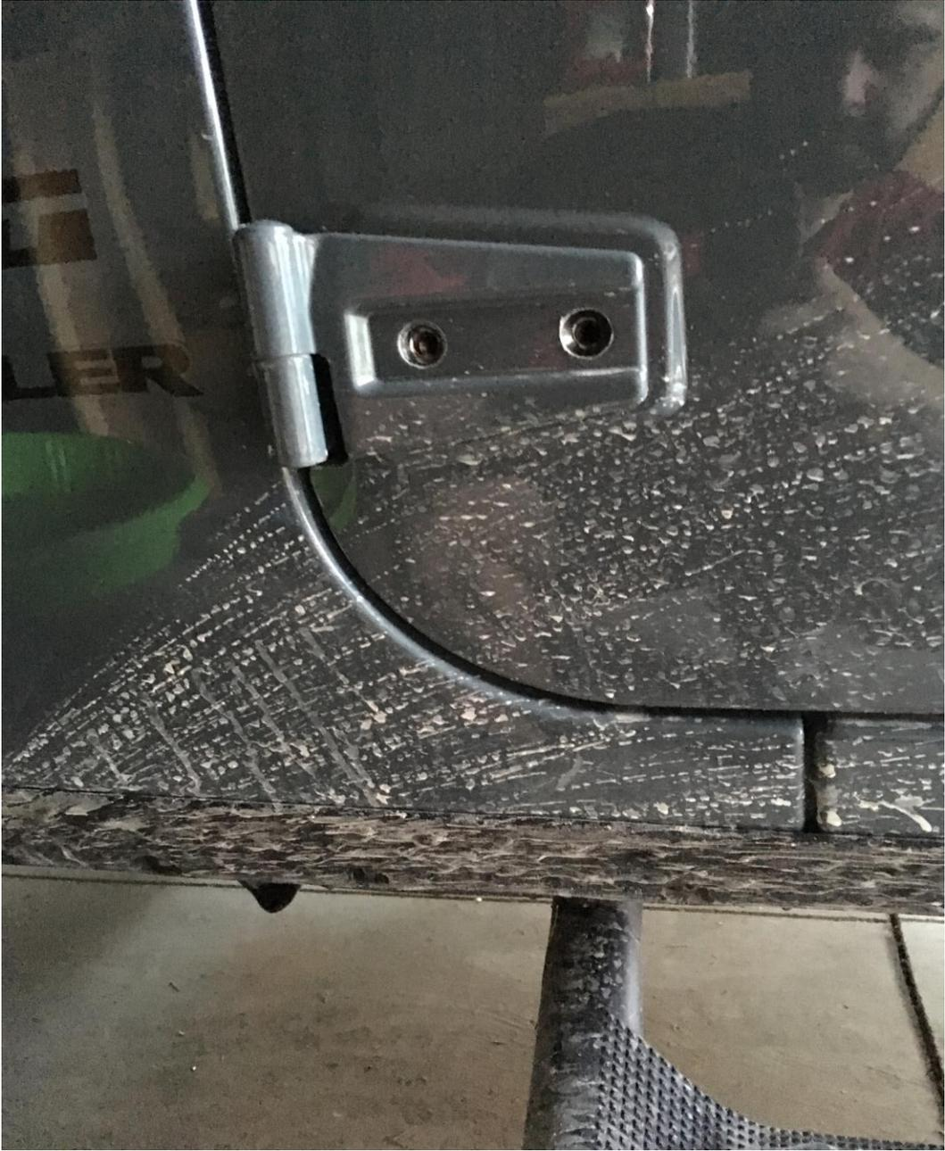
7. Again replace your T-50 Star bit with a T-40 Star bit, place the second (2<sup>nd</sup>) Rugged Ridge door hinge flush over your bottom door hinge and install the two (2) Rugged Ridge door hinge screws with the T-40 Star bit attached to your ratchet.
