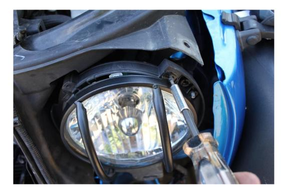
19. The guard is a tight fit so make sure the head lamp is properly aligned and tighten all screws. DO NOT OVERTIGHTEN!
