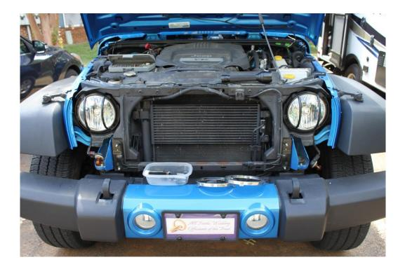
21. Set the grille in place tilted forward and reconnect the parking light/turn signals by twisting them back into the housing.
