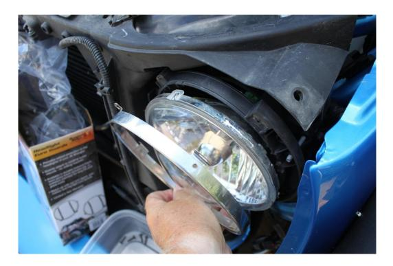
18. The Rugged Ridge Headlight Euro Guards replace the retainer ring. Make sure the headlamp is aligned correctly, (they have locating tabs) and start the torx head screws but do not tighten them until all four are installed.
