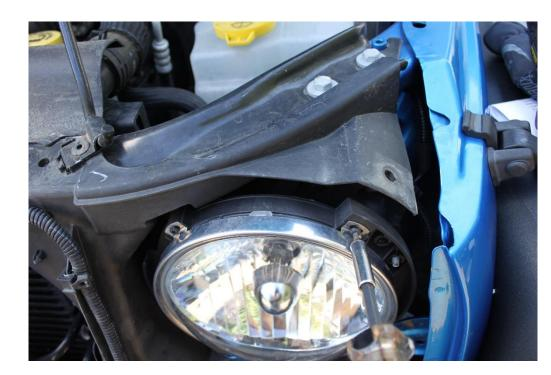
16. Using your Torx bit screwdriver remove the headlight retainer ring screws and remove the retaining ring. Place the Torx head screws in your tray. You will need them to install the guard and they are not easily replaced.
