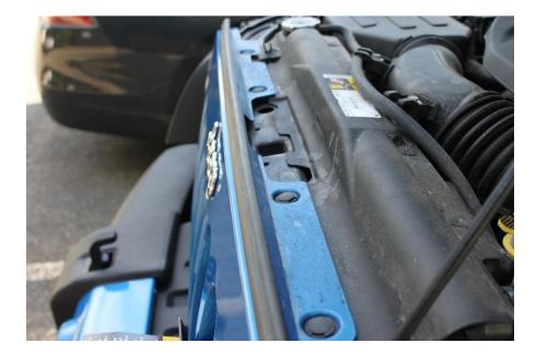
4. With your straight bladed screwdriver gently pry the center of each retainer up.
