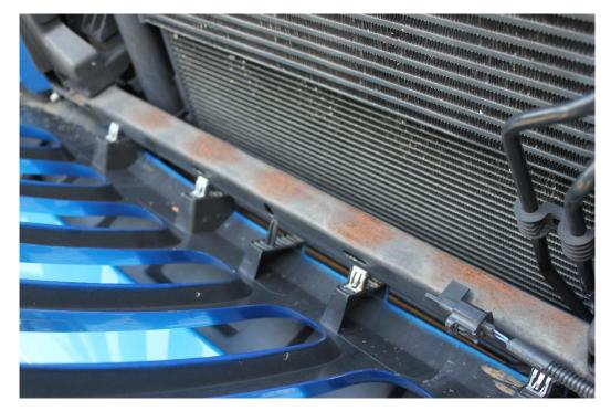
23. Set the grille up and snap back in place. Then make sure the retainers under the headlamps are snapped in.
