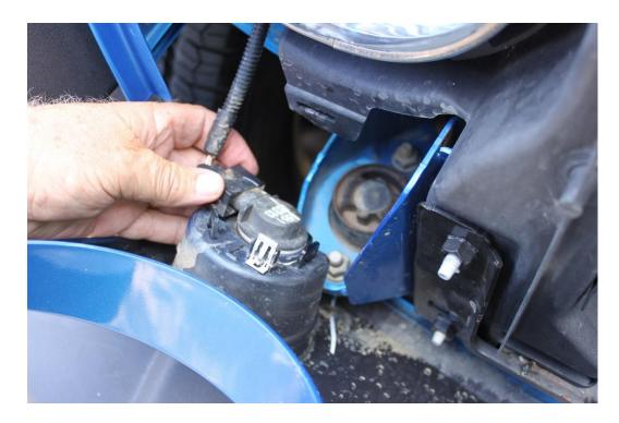
12. Pull the bulb socket out of the housing. Do this on both sides.
