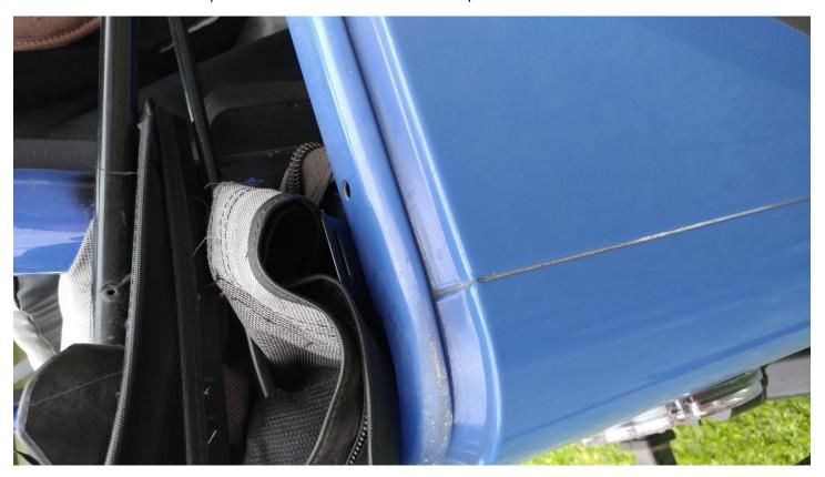
4. Loosely install the rear straps to apply pressure to the front seam.
