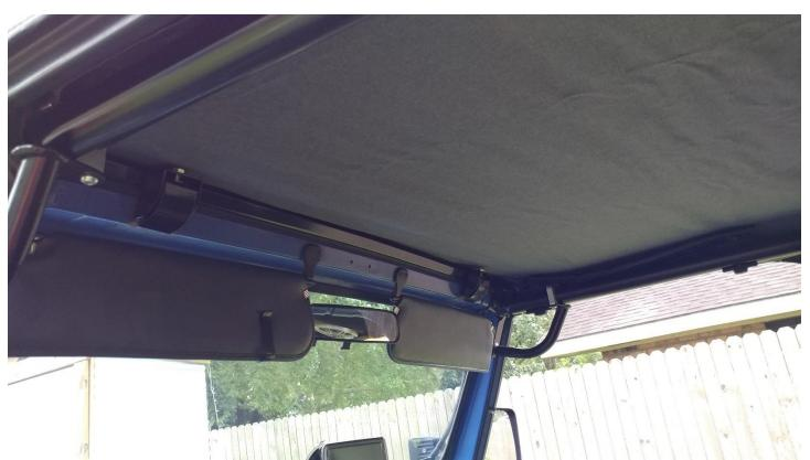
9. Secure the outer straps around the center roll bar.
