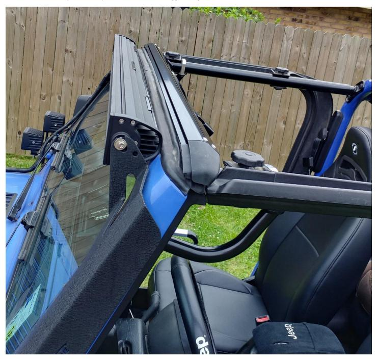
2. Start by laying the Rugged Ridge Roll Bar Top over the roll bars and pressing in the front seam. It will not stay.
