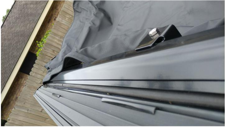
3. Locate and insert the provided hooks. On the rear of the Jeep.
