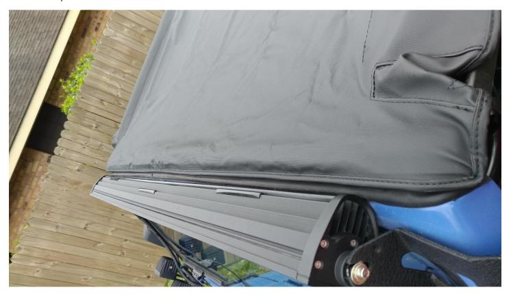
6. Secure the front Velcro straps around the door surround and tuck the plastic portion into the door surround just like the factory soft top.
