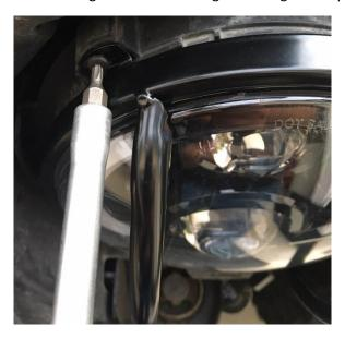
11. Now your guards are installed, and you are ready to reinstall the grill. In reverse order, install the turn signals, and push the clips in place at the bottom of the grill. Next, reinstall the plastic clips at the top of the grill, and close the hood.
