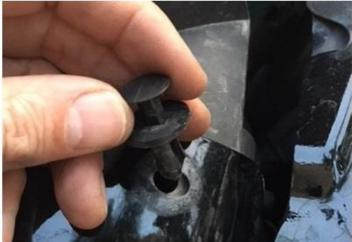
4. Once the clips are removed, gently pull the top of the grill toward the front of the Jeep. There are a series of clips on the inside of the grill holding it in place..
