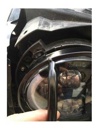
10. Using the T15 Torx again, install the original screws holding the new guard in place.
