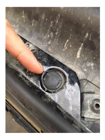
3. With a flathead screwdriver, carefully pry up the head of the clip and gently remove it.
