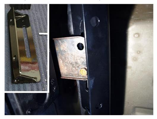
7. Slide the skid plate in place with the angled end facing up towards the front bracket and align the bolt holes. Place a washer on each 16mm bolt that was suppled with the skid plate. Then screw the bolts into each of the front bracket into the skid plate. Do not tighten.
