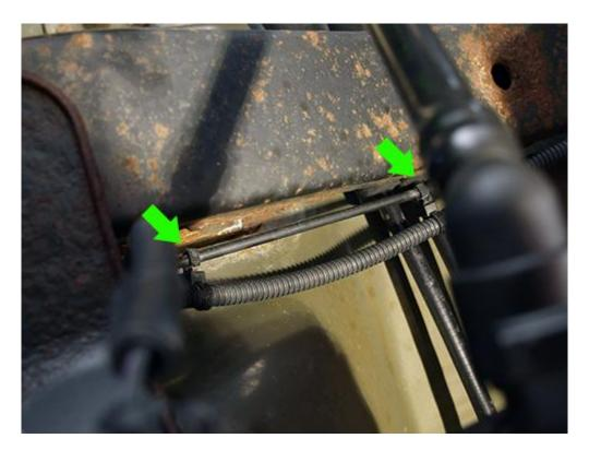
4. Remove both front blots holding the Evaporator and slide the rear bracket from the front to the back. Make sure that the bolt hole of the rear bracket is facing the driver side. Screw one of the bolts back in to hold the front of the Evaporator in place.
