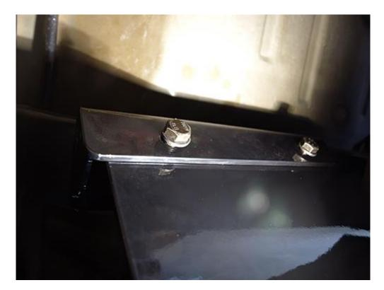
8. Screw the 6mm flathead Allen bolts through the rear of the skid plate into the rear bracket. Tighten the three 16mm factory Evaporator bolts and then tighten all the skid plate bolts. Note that the front Evaporator bolts maybe a challenge to tighten with the socket wrench as the front skid plate bracket now covers them. Use a 16mm wrench or ratcheting wrench to tighten.
