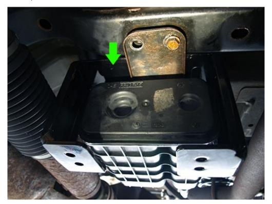
5. Slide the rear bracket all the way to the back of the Evaporator and remove the rear bolt. Align the long hole in the rear bracket with the bolt hole in the Evaporator bracket. Screw the bolt back in to hold both brackets in place. Do not tighten the bolt.
