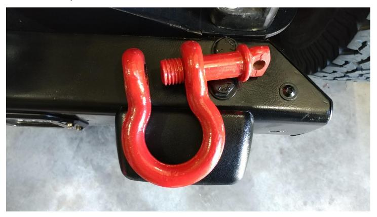
3. Insert the pin with the D-Shackle around the mounting hole
