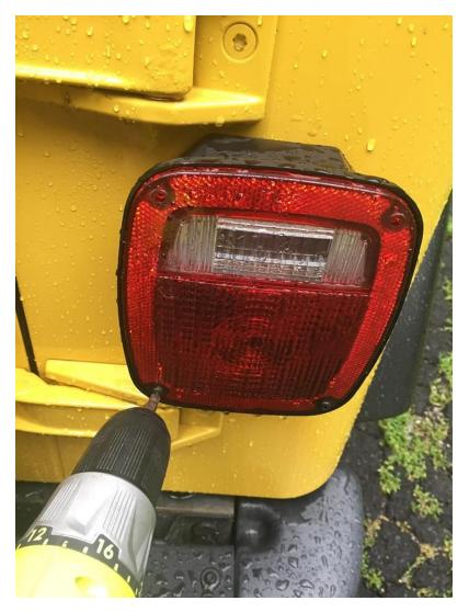
5. Place the stone guard over the tail light and attach the guard. Do NOT over tighten. You could crack the plastic.
