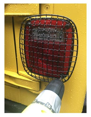
6. Remove the 2 blinker screws with a Torx 15. Put aside and save them. You will use the screws and washers that came with kit to install these. The Torx screws are too short to utilize.
