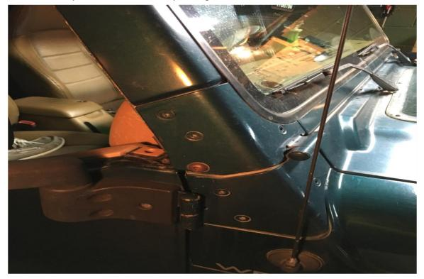
Place passenger upright over hole and align. Insert two of the supplied 6mm bolts and washers. Hand tighten.
