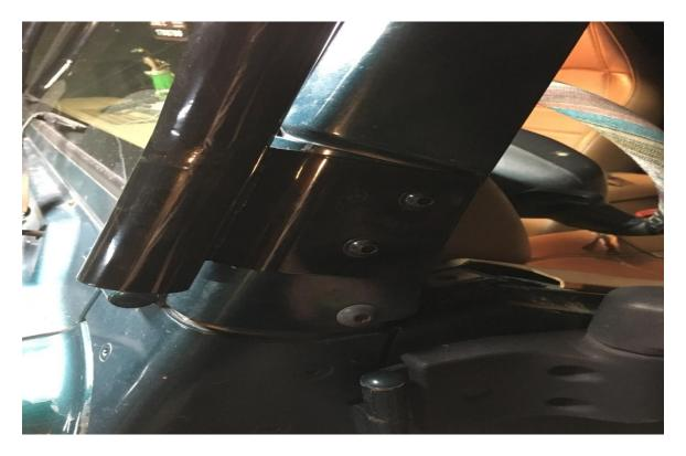
Mount crossbar onto uprights and put Philips screw with washer into hole. Hand tighten
