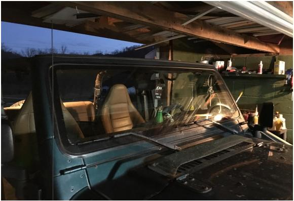
Remove the top two T-40 screws on passenger side of windshield
