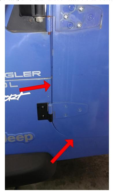
9. You will need to use the door to even out the door gaps. When the gaps are even and the door can close, tighten the provided 3/16 Allen bolts. \*\*Even with the door closed pressure will have to be applied to even out the gaps.
