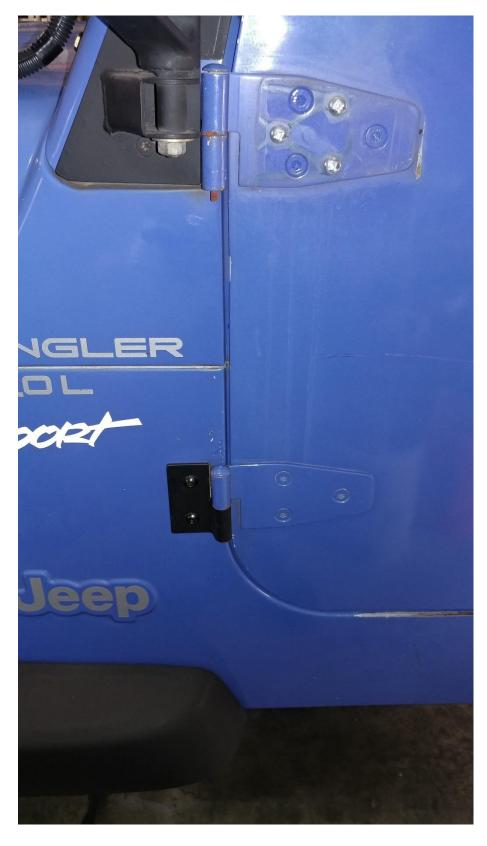
10. After the provided 3/16 Allen bolts are tight installation is complete.
