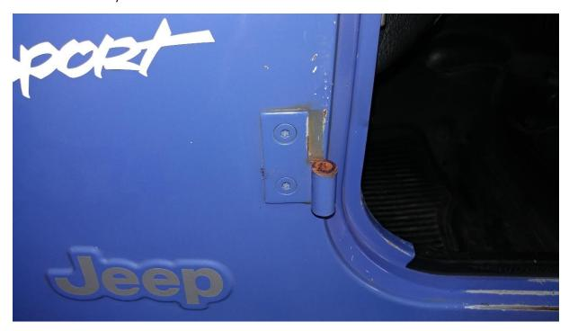
4. The bolts are held in by a backing plate that is not secured to the body. But can be easily accessed, near the door limiting strap attachment.
