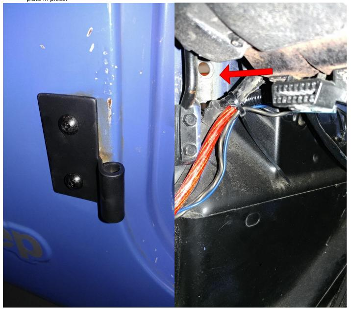
8. Do not tighten the provided 3/16 Allen bolts. Leave them loose and reinstall the door.
