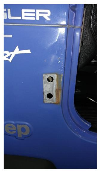
7. Insert the provided 3/16 Allen bolts in the new Rugged Ridge Black Lower Door Hinge. While holding the backing plate in place.
