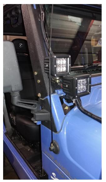
2. Use a 3/8 wrench to remove the factory antenna.
