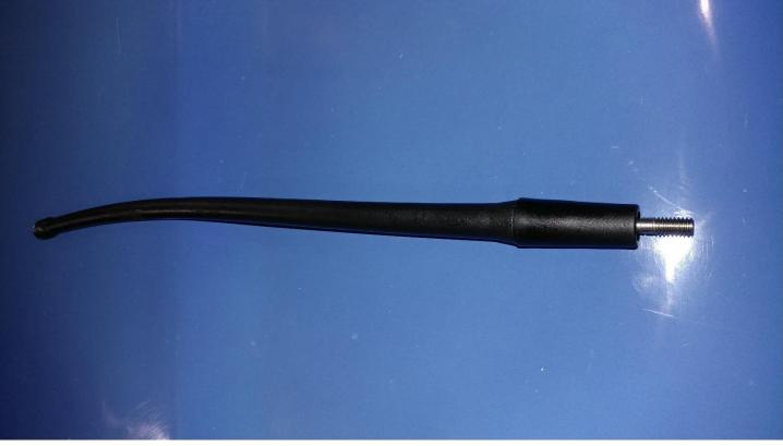
5. Use your hands to tighten the new Rugged Ridge 13 in. Reflex Stubby Antenna. It may have a gape due to the threaded shaft on the Rugged Ridge 13 in. Reflex Stubby Antenna being longer than the factory.
