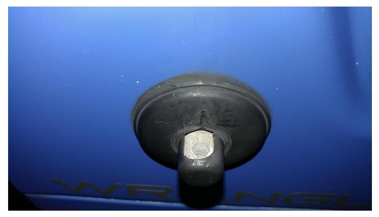
4. After removing the factory antenna I observed that the new Rugged Ridge 13 in. Reflex Stubby has a longer threaded shaft than the factory antenna.
