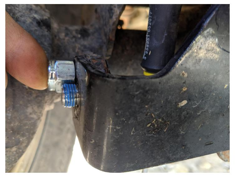
4. Repeat process on opposite side. Insert snap pins to hold links in place. Now verify that link length is equal on both sides and adjust as necessary. In most suspension configurations, ideal length will put your sway bar running "level" or parallel to the frame.
