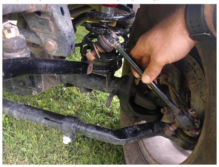
2. Install top stud through sway bar and link and tighten using 19mm wrench and screwdriver or punch through hole in end of stud.
