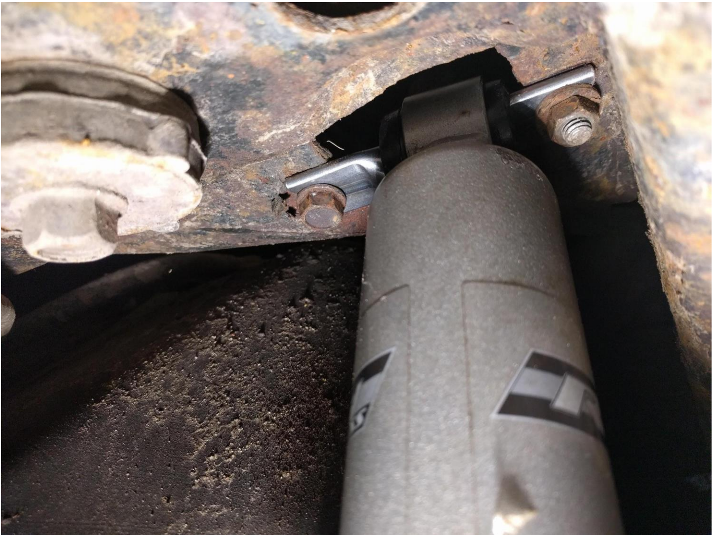
9. Complete installation by reinstalling Lower mount to axle using factory 15/18mm bolt and nut.
