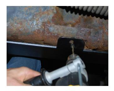
7. Drill two (2) 3/8" holes into the piloted holes in the mounting bracket, using a drill stop to avoid drilling too far. Again, be careful not to drill too far, to avoid causing damage to the gas tank.
