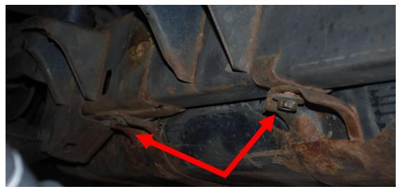
4. With the help of a friend and a floor jack, position the new skid plate, with logo toward front of vehicle, so bolt holes are aligned. Reinsert the four (4) original bolts in the front and sides, but do not fully tighten yet.
