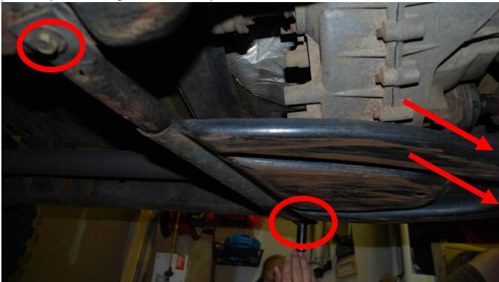
3. Using the 18mm socket, remove the front two (2) gas tank mount bolts, then remove the two (2) side bolts. Save these bolts, also.
