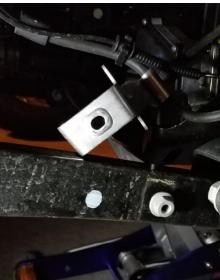
2. With a 21mm socket and a 24mm wrench, remove the lower control arm bolt attaching the arm to the axle and the frame (Passenger's side shown). Keep the factory hardware in the frame and axle as it will be reused.
