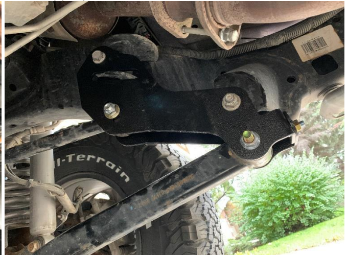
Passengers Side Bracket Installed
