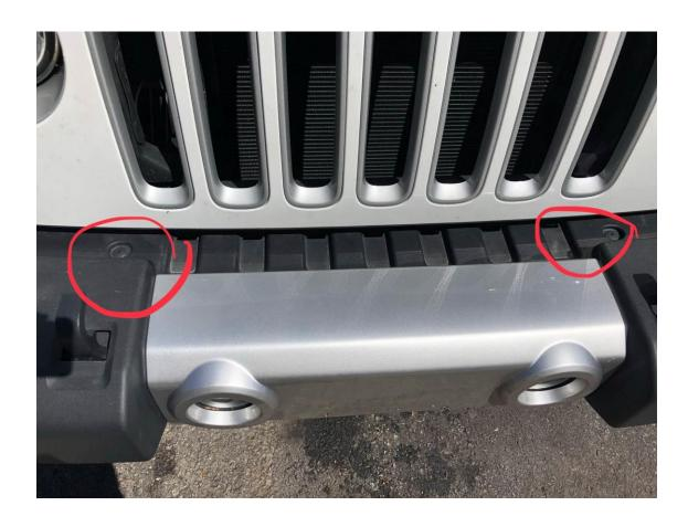
4. Disconnect fog light wiring from lights. These can be accessed easily from under the bumper. Remove the 8 nuts connecting the bumper to the frame. Some of these can be accessed from above while others will need to come from below.
