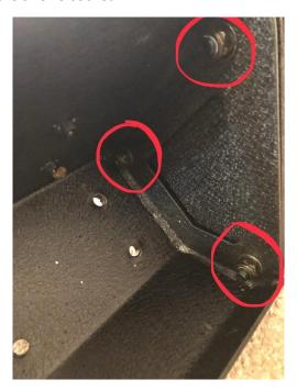
2. Remove the flat end pieces and replace them with the stubby bumper ends; the open portion of the stubby bumper end should align with the underside of the bumper. Place the washers then the nuts on each bolt. Hand tighten all 3 nuts before using the size 19 socket to finish. Repeat for the other side.
