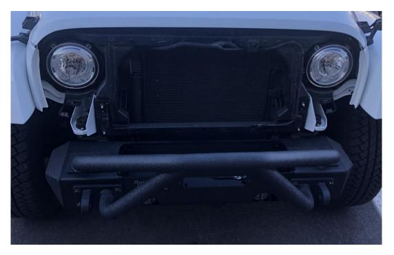
10. Reconnect fog lights to wiring harness, zip tie wires as needed, and re-insert front grill by pushing back in until all tabs are popped in place. Then re-insert pop tabs at the top of the grill and reconnect turn signals.
