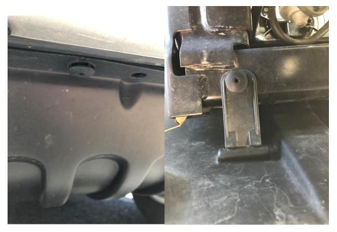
3. Remove the plastic screws connecting the upper liner to the front bumper. These screws strip easily and may need to be drilled out.
