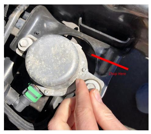
7. Attach provided bracket hardware as shown. Remove cable ties attached to vacuum tubing within engine block to allow movement of the pump. Position as shown below and drill hole with 1/4" bit. Spray hole with rust-preventing paint and remount vacuum pump.
