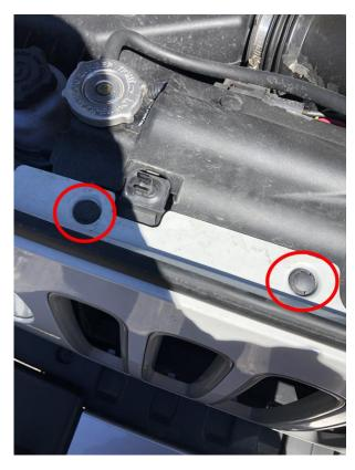
2. Remove pop tabs for plastic front skid plate located under the front bumper. One set are located directly under the bumper at the front, while the others are connected to the metal frame underneath.
