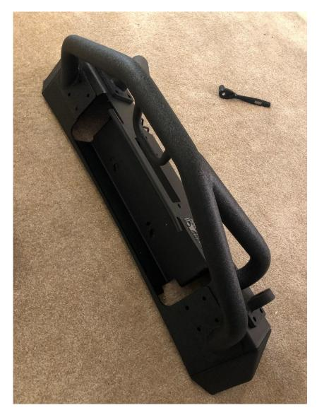
5. Insert all 8 bolts and washers hand tightening only. Once all bolts are inserted, completely tighten all of them with the size 13 socket.
