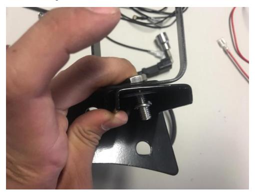
3. Attach the included nut onto the screw and tighten with a % " socket.
