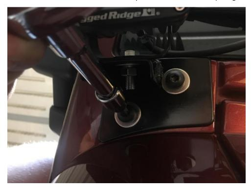
8. Remove the two cowl torx screws with a T27 Torx bit.
