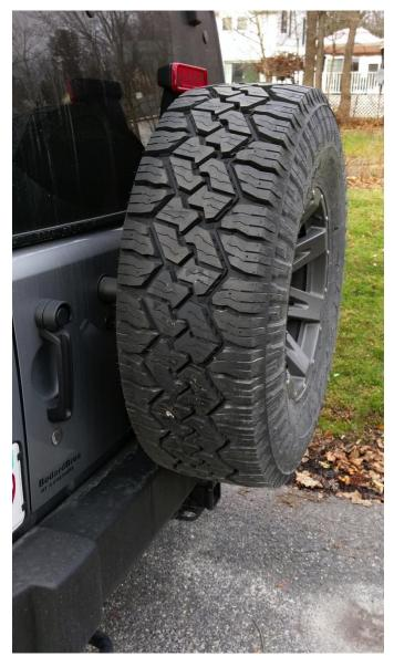
Note that before install with new oversized tires and wheels with appropriate offset that the tire is hitting the bumper slightly and needs to be raised quite a bit (hence the need for the upgraded part). I found it helpful to measure mounting surface and height of the stock carrier before install for reference. The new mount raises the tire  $\sim$  3 inches. This will clearly leave room for 37's if/when the time comes.
