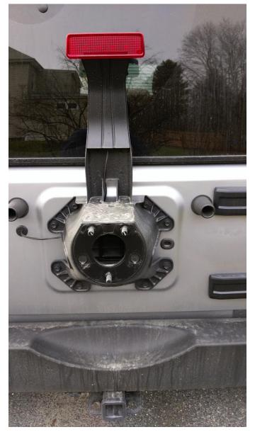
2. Open the tailgate and remove the 3<sup>rd</sup> brake light from the tire mount by removing the (4) T20 torx screws.
