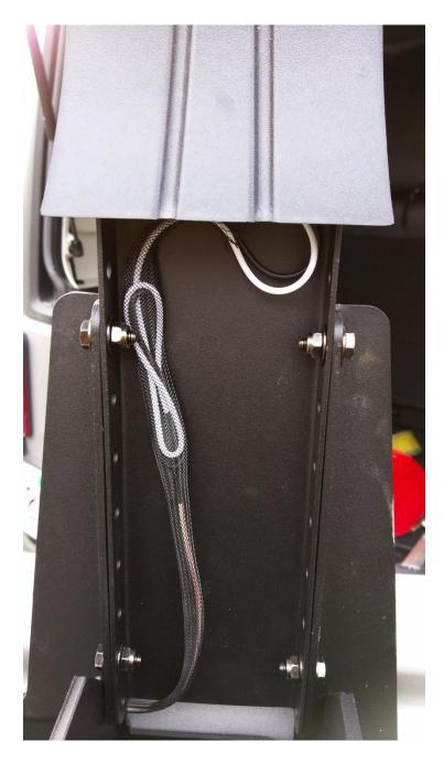
22. Using supplied Phillips screws install the 3<sup>rd</sup> brake light into the extension bracket. The 2 longer screws are for the top, the two shorter screws for the bottom.
