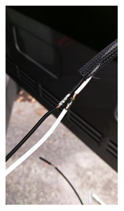
20. Slide shrink tube over newly soldered connections and apply heat to shrink/lock in place. *Use care not to heat the OEM cable sleeve.*
