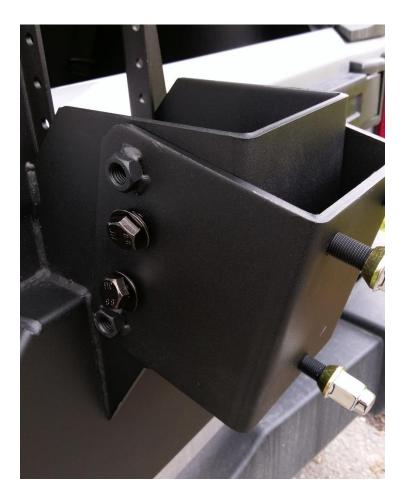
8. Insert the set screws into the welded nuts on the lug plate assembly, do not fully tighten yet.
