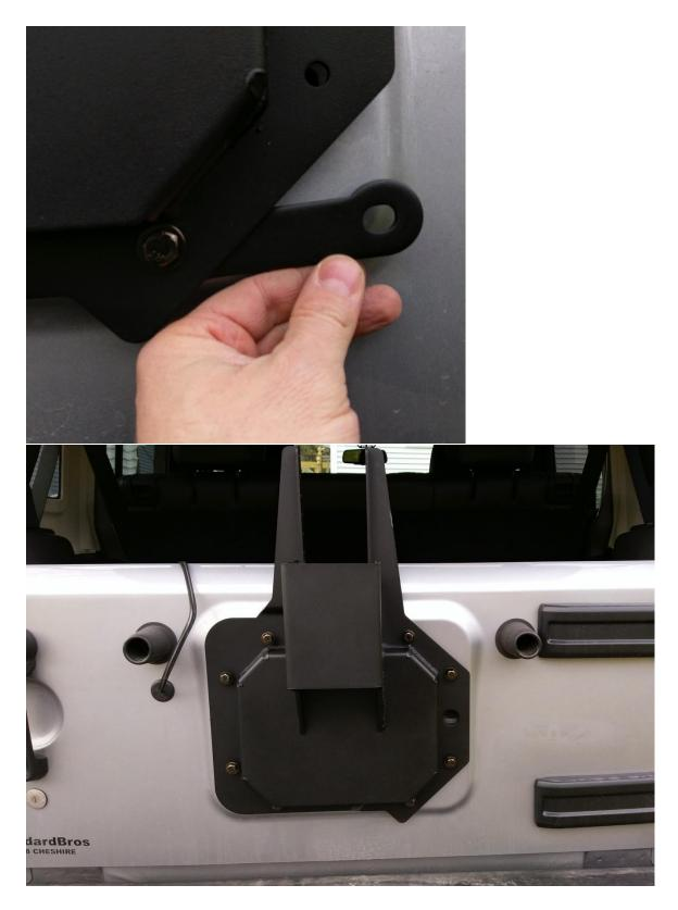
7. Slide the lug plate assembly onto the mounting plate assembly and loosely secure with the supplied M12 hardware. Do not fully tighten yet.
