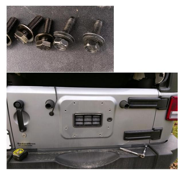
5. After cleaning mounting surface on the tailgate. Set the new tire carrier plate assembly in place loosely threading 4 of the supplied M8 bolts and washers *on the left side of the mount. They are installed loose on this side so that you can install the spacers on the right (assuming you are not using the RR Spartacus Hinge Assembly (separately purchased).*
