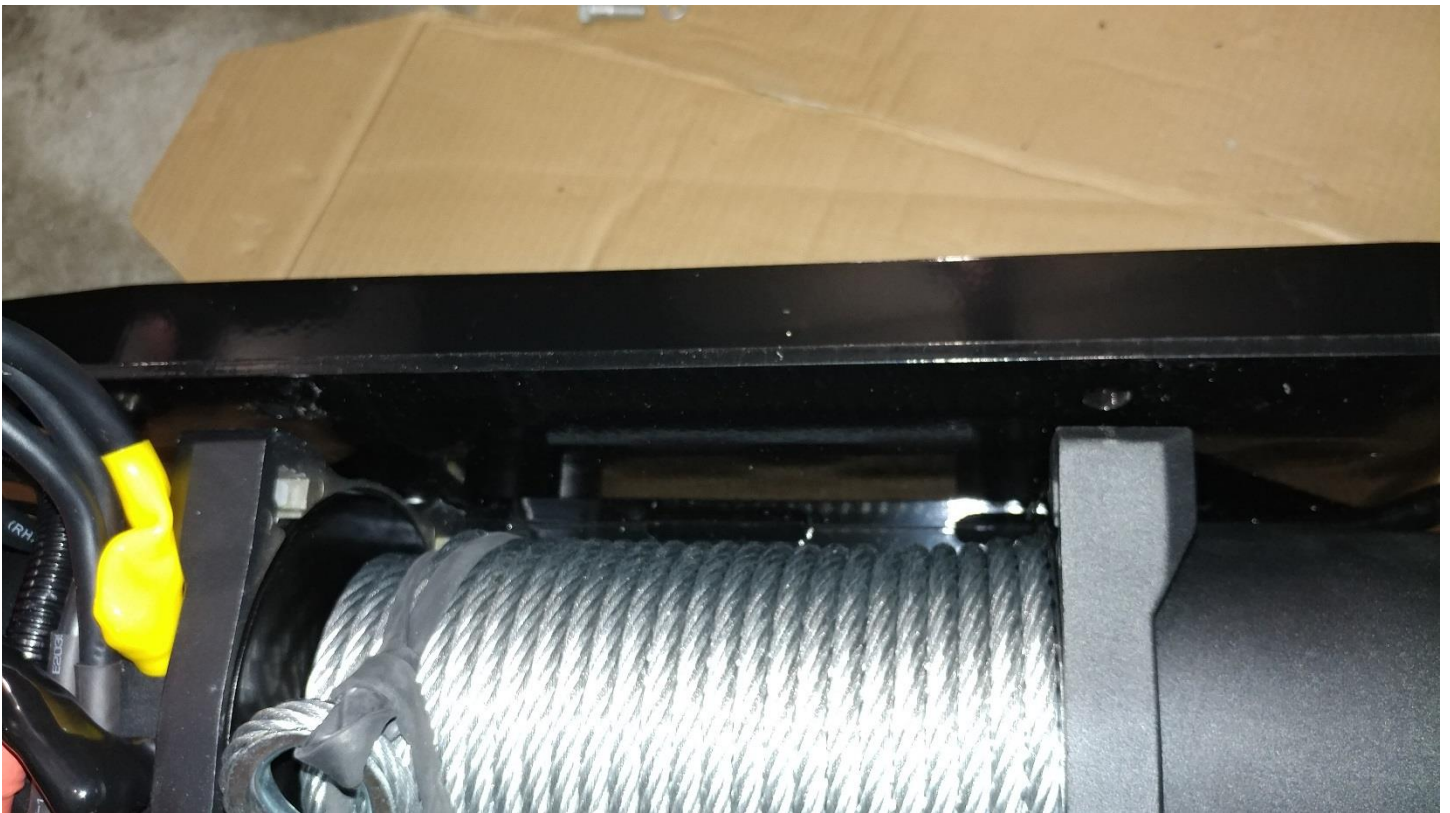
14. Mount the winch to the winch plate using the provided 16 mm bolts
