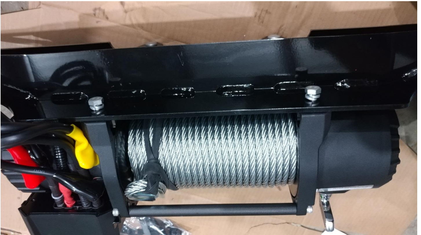
15. Cut the rubber band holding the cable in place.
