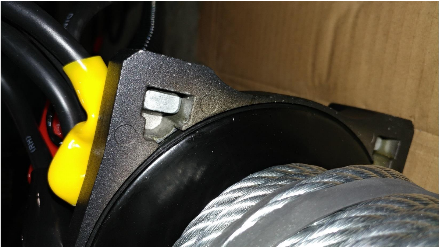
14. Mount the winch to the winch plate using the provided 16 mm bolts
