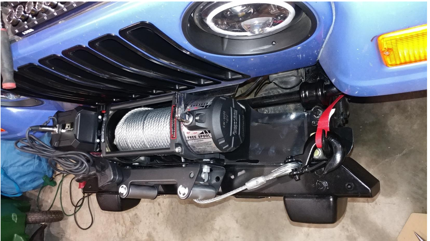
18. Mount the winch plate to the frame rails, using the factory bumper bolts (19 mm) and sway bar bolts (16 mm)
