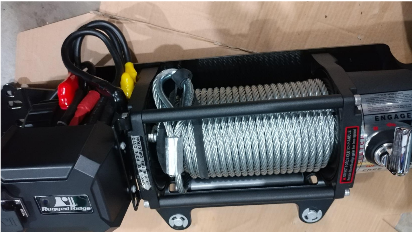
15. Cut the rubber band holding the cable in place.
