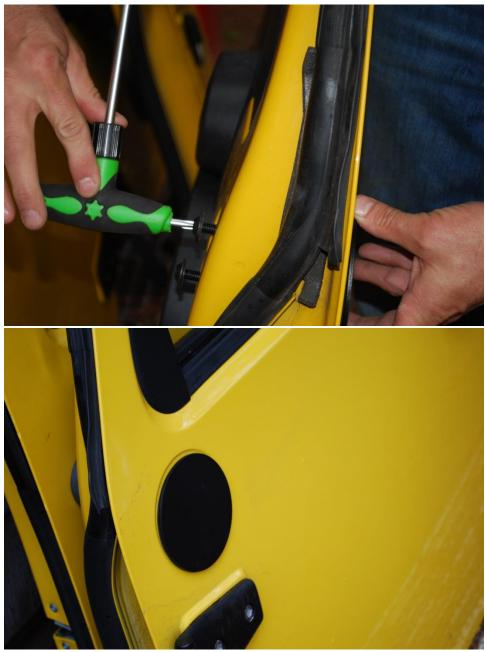
9. Using the T40 Torx socket and ratchet, remove the bolt from the bottom of the mirror. These bolts are VERY tight and if there is any corrosion they may be difficult to remove. Starting it while the mirror is still on the door may help, but that would add risk of damaging the door. If you cannot remove this bolt, ExtremeTerrain.com sells a selection of replacement mirrors at reasonable prices. Retain this bolt.
