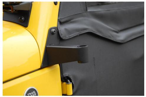
5. Moving to the factory door (in the images, it was removed from the vehicle, but that is not necessary), remove the two mirror mounting bolts on the inside of the door using the T40 torx socket and ratchet. Retain the bolts.
