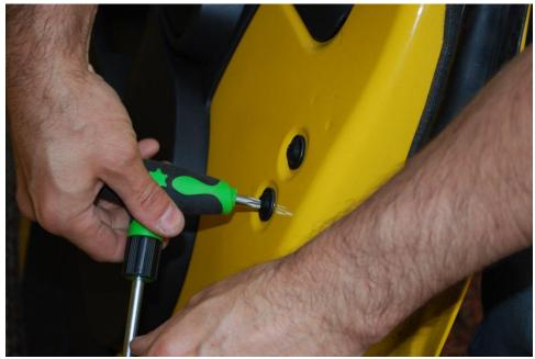
6. Carefully remove the mirror. The base may be stuck to the door, just gently pull and it will come free. In the images, you will notice that the mount for the mirror being removed is highly corroded (the white powder). This is a sign that your mirrors may not come apart in a subsequent step.
