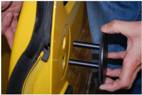
8. Reinstall the bolts removed in step 5 to hold the plate in place. Tighten these bolts gently. The specification is 15 ft-lbs., but be careful not to overtighten and deform the door.
