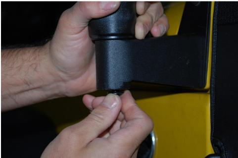
13. Test the ability to fold in the mirror. If the mounting bolt turns with the mirror, tighten the bolt more. Repeat until you can fold the mirror in without the mounting bolt turning with the mirror.
