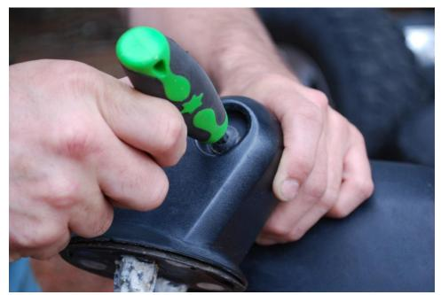
10. Separate the lower mirror bracket from the mirror head. The mirror head is pressed into the base, you may have to partially reinstall the bolt and tap it with a hammer to get them to separate. You may notice that the mirror in this picture is new – the original from this vehicle was too corroded to save.
