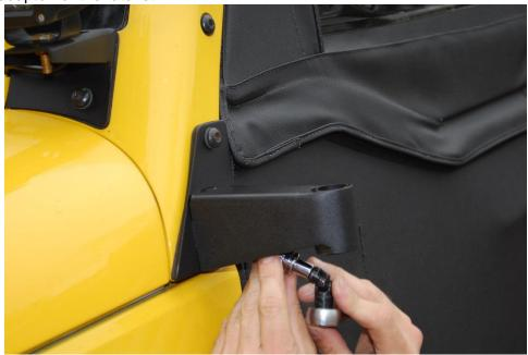
4. Align the bracket so the lower edge is parallel to the lower edge of the A-pillar and the upper edge of the fender and tighten the bolts using the T40 torx socket and ratchet to 15 ft-lbs.
