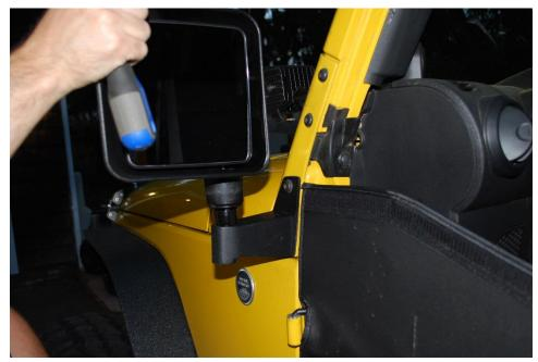
12. Using the bolt from step 9 and the T40 Torx socket and ratchet, attach the mirror head to the relocation bracket. Tighten the bolt to 15 ft-lbs.
