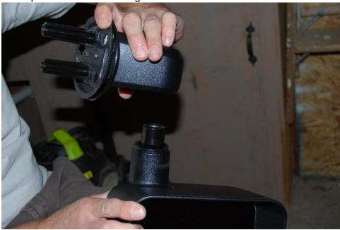
11. Place the mirror head in the relocation bracket.
