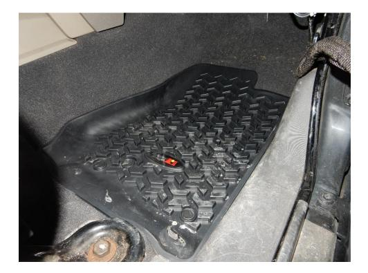
8. Position the rear floor mat so that the cut-outs for the rear seat supports are up and the tread pattern is facing the front of the vehicle.
