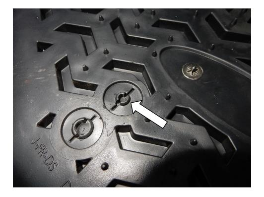
4. Align the new floor mat into place, and engage the point of the floor retainer hook by pressing firmly on the floor mat just beyond the point of the hook.
