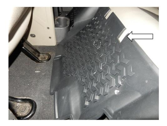
9. Slide the floor mat down into position so that the raised portion of the mat is seated over the front seat mounting bracket.
