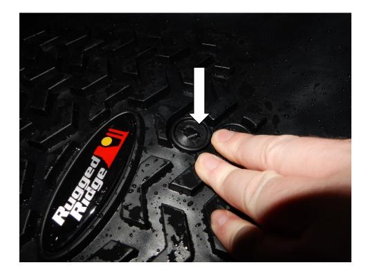
5. Engage the remainder of the engagement hook by pressing firmly on the floor mat just beyond the body of the retainer hook.
