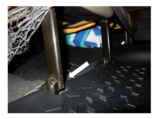
11. Position the cargo floor mat into place with the Rugged Ridge logo toward rear of the vehicle.
