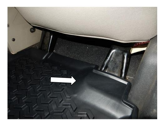
10. Ensure that that the cut-outs for the rear seat supports are aligned with the supports, and that the mat is seated firmly on the floor.
