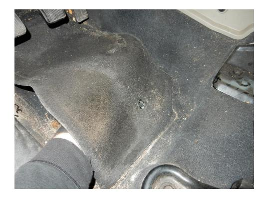
2. Align the new floor mat into position and locate the floor retainer hook below the mat to determine the appropriate retainer hook slot for your particular install.
