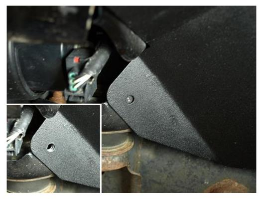
10. Paint the bare metal of the hole with touch up paint and place a 6mm Clip Nut on to the body mount once paint is dry.
