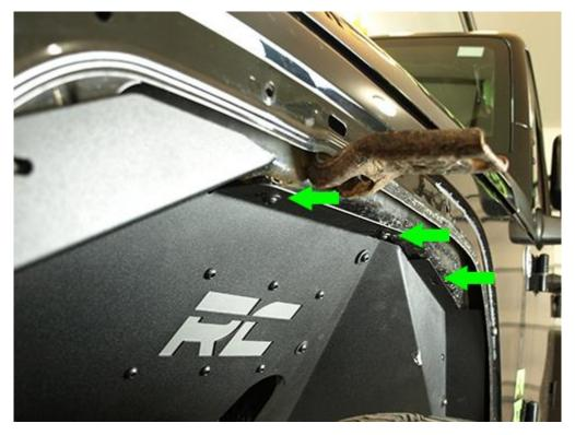
8. Secure the back of the Middle Inner Fender liner to the Rear Fender Bracket using four (4) 6mm bolts and washers and tighten all 6mm blots with 4mm Allen.
