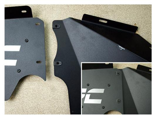
5. Place four (4) 6mm Clip Nuts on the Rear Fender Bracket where the orange arrows are pointing to below. Then place three (3) 8mm Clip Nuts on the opposite side where the blue arrows are pointing to below. NOTE: The clips nuts need to be facing the same direction as pictured. Use a flathead/standard screwdriver to slide the clip nuts off if placed on the incorrect side.
