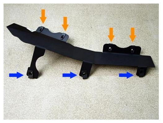
6. Slide the Rear Fender Bracket behind the outer fender with the three (3) 8mm Clip Nuts. Secure in with three (3) 8mm bolts and washers and tighten with 6mm Allen.
