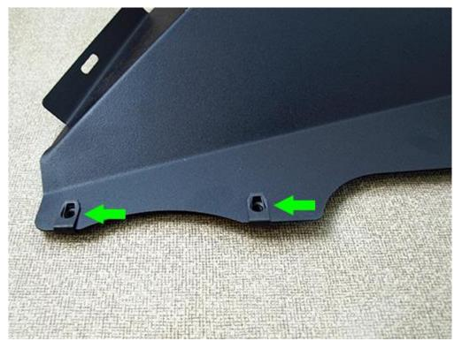
4. Slide the Middle Inner Fender liner behind the Front Inner Fender liner and loosely attach with two (2) 6mm bolts and washers.
