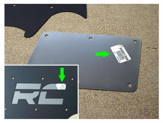
2. Place one of the Back Plates behind the Front Inner Fender liner and secure with six (6) 6mm bolts, washers and Nylock Nuts. Tighten these bolts using a 4mm Allen and a 10mm wrench. *Side Note: You could paint the Back Plate a different color for a custom look.*
