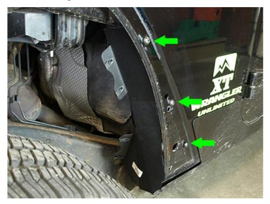
7. Slide the Front and Middle Inner Fender liner behind the tire and into the wheel well. Loosely secure the top of the liner using three (3) 6mm bolts and washers into the factory 6mm Clip Nuts.
