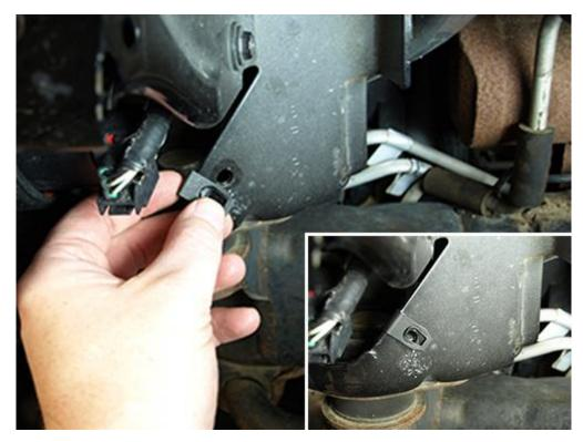
11. Secure the front of the Front Inner Fender liner using two (2) 6mm blots and washers and tighten with 4mm Allen. Make sure that all bolts are tight.
