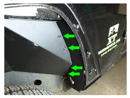
9. Drill a 5/16 hole through the Front Inner Fender and through the body mount of the Jeep<sup>®</sup>.
