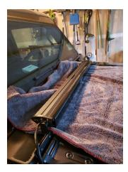
17. Using the hardware provided attach one side of the light bar to the bracket loosely. Make sure the locking washer goes first, then the bracket, then the spacer, then the washer. Repeat in the other side.
