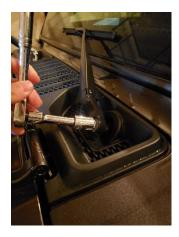
3. Flip the wiper blade away from the windshield after unbolting. This will help release the tension against the bolt and facilitate the blade removal. You might need to use a wiper removal tool or an alternative method.
