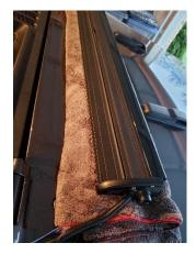
13. Lay the cowl cover back in place and press in all the 12 clips. The fit will be tight. It is advised to start in the driver's side by insert the wiper screw in the cowl cover and then slide in behind the lower portion of the bracket.
