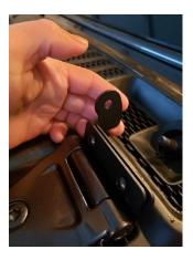
15. Reinstall the windshield wipers, tighten using a 15mm wrench and put the plastic cap back on top of the wiper blade nut.
