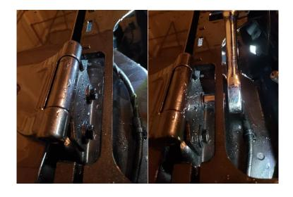
7. Slide in the lower portion of the mounting bracket ensuring that the bend on the bracket points towards the windshield. Tight the bolts and repeat in the other side.
