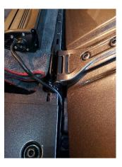
11. Leave a little slack and slide under the foam cover that is inside the hood.
