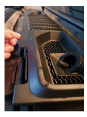
14. Place the top portion of the bracket with the round light bar mounting point aimed towards the inside (driver's side shown). Make sure the top portion of the bracket is installed behind the lower portion of the bracket. Now loosely secure using the provided hardware (70048BAG1). Repeat on the other side.
