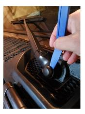
2. Using a 15mm socket, remove the nut.
