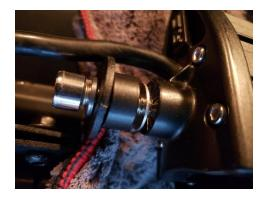
18. Using a 4mm hex key and a 10mm wrench, tight down the bolts on the brackets.
