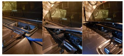
6. Using the 13mm socket, loose the two bolts holding the hood hinge behind the cowl cover. Do not fully remove the bolts, you will only need a small separation of the screw head and washer to slide the lower portion of the mounting bracket in.
