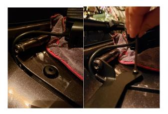
5. Using the 45mm Torx bit and the ratchet, tight the screw in the windshield hinge.
