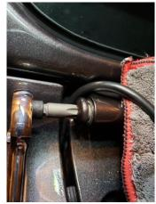
4. Place the rubber spacer provided in place of the Torx screw that came with the JL. Then slide in the bracket in the windshield hinge and secure using the provided bolt.
