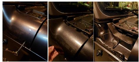
2. Put the towel on top of the cowl and place the light on top of it. Tuck the cable near the windshield hinge and leave the connector reachable from the hood.
