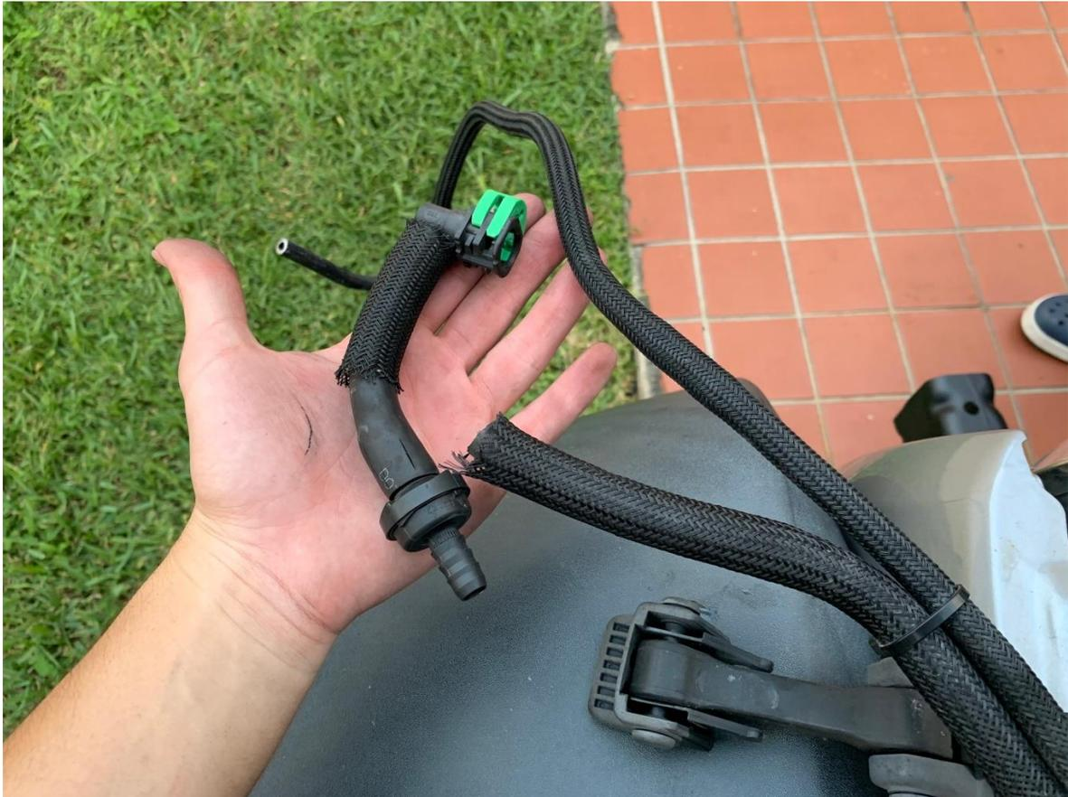
7. Connect the adapter back to the disconnected hose in the engine bay from the previous step. Plug in the other end into the vacuum pump and slide the green tab back into place to secure the hose onto the vacuum pump.
