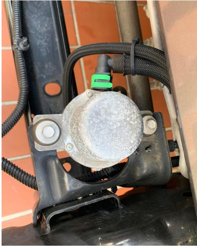
2. Pry up on the tips of the green tab and slide it out, then disconnect both hoses from the vacuum pump. Lastly, disconnect the wire harness.
