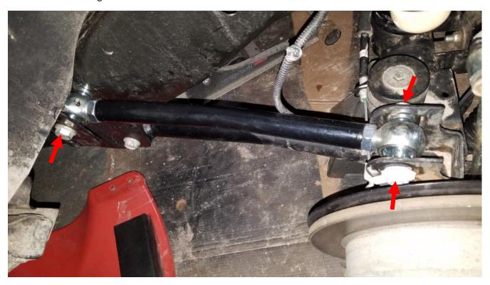
12. On the driver side, you will be able to see where to place the frame side flag nut by looking through the view hole as shown below. Notice at the top there is a small slot for the tab to slide into. Using this view hole, align and tighten the driver side flag nut. Then repeat on the passenger side, but you will not have a view hole to help line it up so be patient and align it by feel.
