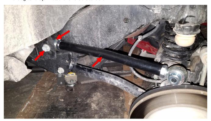
**7.** Using the control arm from step 6, adjust the other control arm to the exact same length. Then apply red Loctite to all 4 jam nuts.
