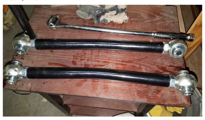
**8.** Now you will need to tighten the jam nuts to 200ft/lbs. I recommend having a friend help you. Using a large screwdriver or long socket extension, hold both joints straight. Using a 1 5/16" crowfoot and torque wrench, tighten the jam nuts. Make sure you do so while holding the joints as straight as possible. Do this for both control arms.
