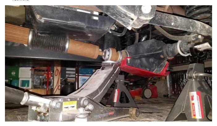
**4.** Use a 21mm socket to remove the driver side control arm bolts, then remove the control arm. Remove both bolts and both flag nuts, then remove the control arm. Repeat this step on the passenger side.
