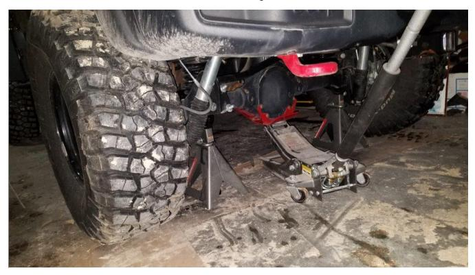
**3.** Place a jack where the driveshaft connects to the differential as shown. Lift the jack just enough to support but not lift it.
