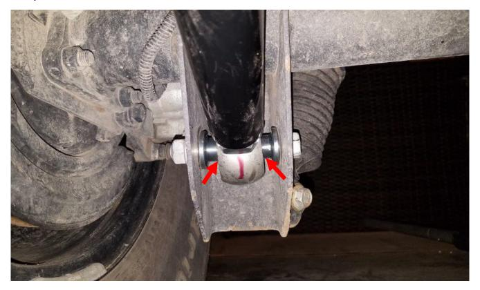
**11.** Now install both control arms. Install the factory bolts and flag nuts as shown. See step 12 for more details on the frame side flag nut.
