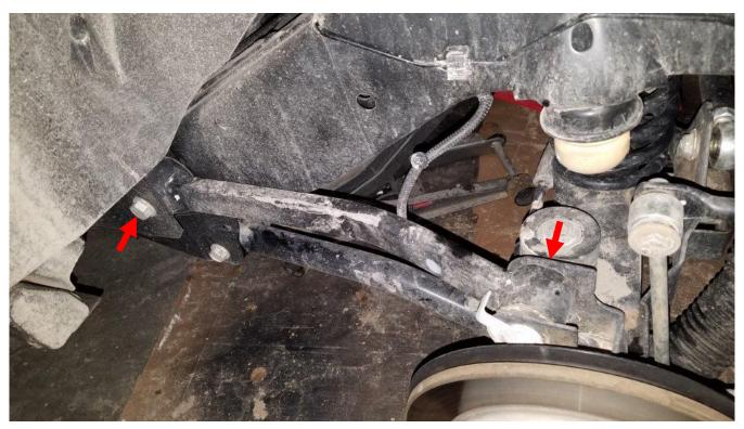
**5.** Now using the jack supporting the front end of the differential, lift it until the pinion is aligned with the driveshaft. Use an angle finder placed as shown below to ensure both angles are equal or at least within 1-2 degrees. Note: This type of driveshaft alignment is best for the stock CV driveshaft. If you have an aftermarket driveshaft, align it using manufacturer instructions.
