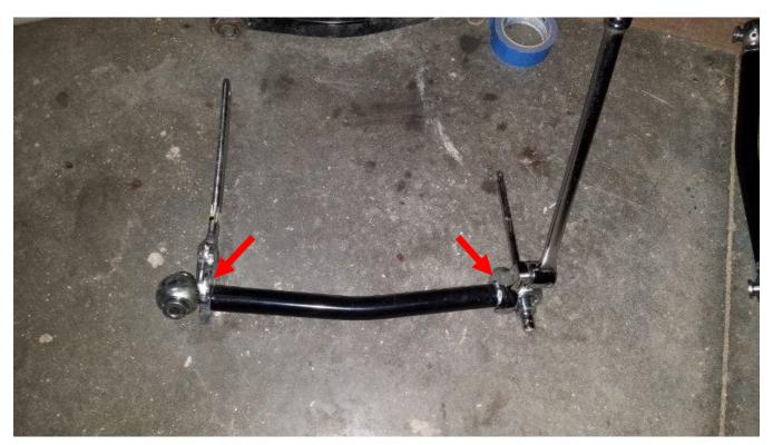
**9.** Then use a 7mm socket to install the 4 grease fittings. Be careful not to overtighten them. I also recommend greasing them while you're at it. Use only 000 grade grease for Rock Krawler joints.
