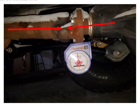
**8.** When you find the proper length you will need to tighten the jam nuts to 250ft/lbs. I recommend having a friend help you. First, apply Loctite to the threads, then using a large screwdriver or long socket extension, hold both joints strait. Using a 1 ½" crowfoot and torque wrench, tighten the jam nuts. *Note: If your wrench will fit you can also tighten the jam nut with the control arm still on the vehicle.*
