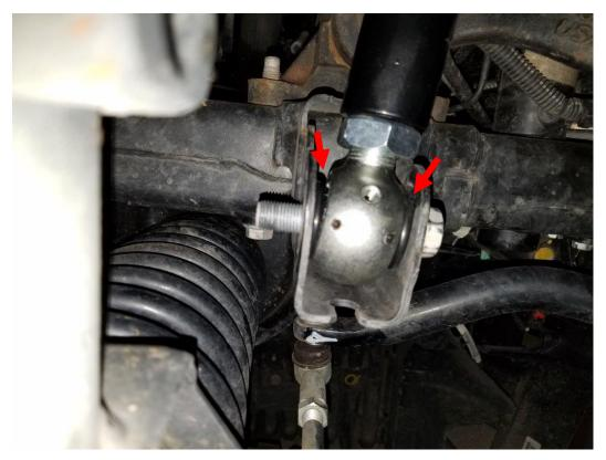
**11.** Last, be sure to tighten all 4 control arm mount bolts. Using 2x 21mm sockets and a torque wrench, tighten them to 125ft/lbs.
