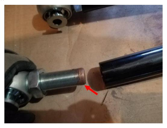
2. Using a 7mm socket install the grease fittings on all joints. Be careful not to overtighten them as they can easily strip. Using 000 grade grease, grease all the joints while you're at it.
