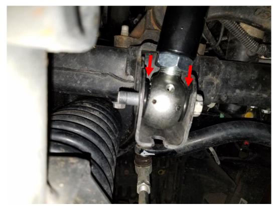
**9.** You want the joint to be aligned as shown below. But you also want the grease fitting to be pointed up, NOT as shown. Hand tighten both jam nuts to keep the ends in place. Then remove the track bar to tighten the jam nuts.
