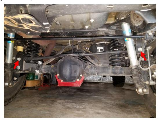
**2.** Before installing the track bar, spread a small amount of grease on the heim joint spacers. This will help hold them in place while you work, and prevent corrosion.
