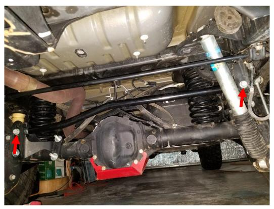
7. Now you need to determine if your track bar is the correct length, and has centered your axel. Measure the distance from the fender to the outer edge of the tire. You can also measure from the frame to the inside of the tire. Measure at the same point on both rear tires and compare. If needed adjust the track bar length so that these measurements match. A longer track bar will push the left wheel out further, and a shorter track bar will push the right wheel out further.
