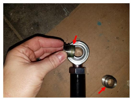
**3.** Unscrew both ends and apply a small amount of anti-seize to the threads, then crew them back in. This will help make sure it is still easily adjustable years down the road.
