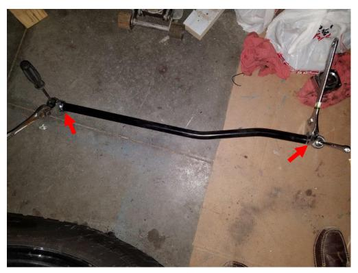
**11.** Using a 7mm socket, screw in the grease fitting. Be careful not to overtighten. The joint is supposed to come pre-greased, but I recommend putting some in it just to be sure. Use a grease gun with 000 grade grease.
