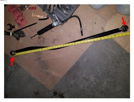
**6.** Now insert your track bar as shown. The bend should be above the differential as shown. Insert the bolts in each side but do not tighten.
