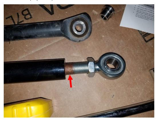
**4.** Then be sure to apply a good amount of red Loctite to the jam nut threads.
