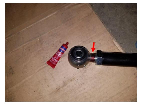
5. Next, adjust your new track bar to the desired length. This will depend on your lift height and track bar bracket. RK recommended starting lengths: 1.5" lift – 39 11/16", 2.5" lift – 39 3/4", 3.5" lift – 39 3/4". Depending on your lift height, choose your desired length and adjust the ends of your new trackbar. The measurement is taken from the center of each mounting hole. Then hand tighten the jam nuts to keep the ends from moving too much.
