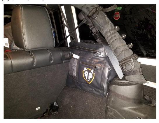
**4.** Using the attached straps, route the top front strap over the roll bar, and the top rear over the seat belt bracket as shown and tighten the straps as necessary. Make sure the strap does not interfere with seat belt operation.
