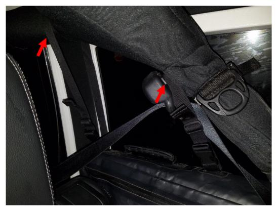
5. Use the rear strap to wrap around the roll bar base as shown, and tighten.
