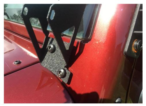
5. Take the T40 Torx bit and tighten the screws lightly.
