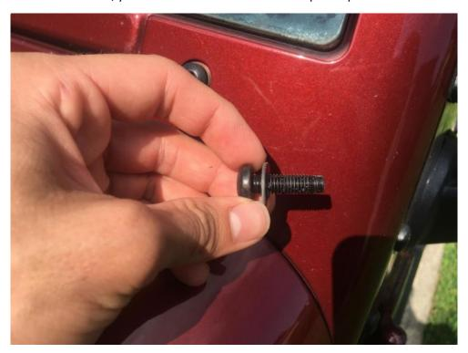
3. Insert the screw into the holes of the bracket, then screw the plastic piece back onto the screw. Make sure to screw the plastic piece onto the screw completely, until it touches the metal bracket.
