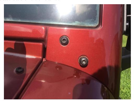
2. Once the screws are removed, you will have to unscrew this small plastic piece from the screw.
