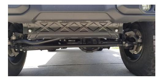
**Step 3:** Next is removing 2 clips that hold the filler panel between the bumper and grille. To do this again use the flathead screwdriver or pry bar to pop the clips out.
