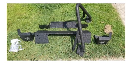
**Step 7:** I laid out all of the hardware to make it easier to find and keep organized during the assembly process. There is a lot more hardware included than you will be using to install the bumper so don't freak out when you have some left over as these are for mounting winches and other pieces to the bumper later.
