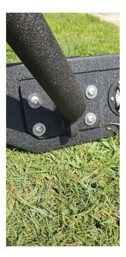
**Step 8:** `Next you will install the 2 end caps to the main body of the bumper. You will need the T30 Hex bit and the 13mm socket for this step. Each end piece has 3 bolts that need to be installed. You will you the Bolt #6, Washer #14, and nut #11 for each of these 6 holes.
