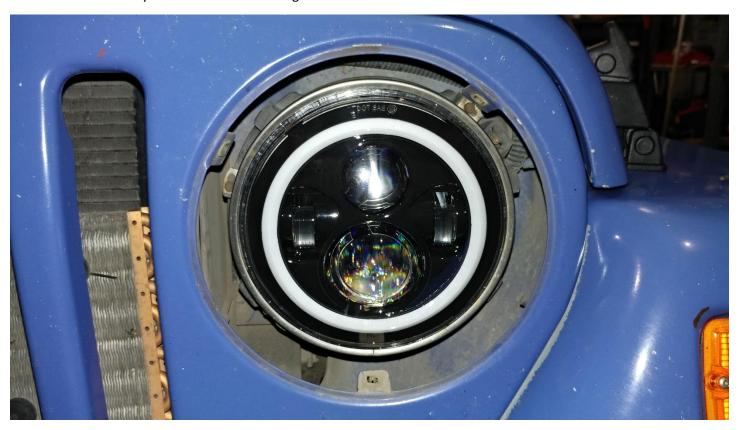
4. Using the factory bezel to determine which RedRock 4x4 Matte Black Headlight Bezel needs to be installed on the driver or passenger side. Insert the correct bezel into the Jeep grill.
