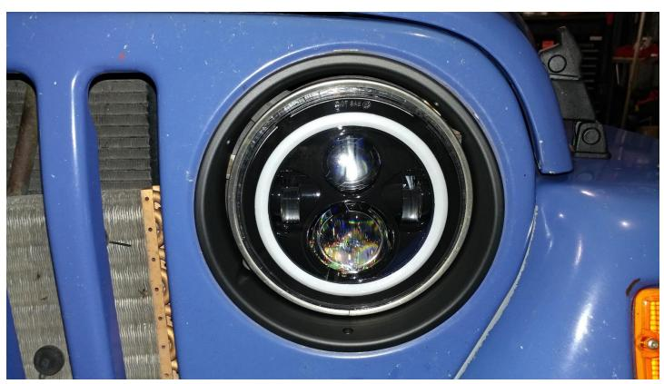
5. Reinstall the 3 – T15 start screws. The backing for the screws is plastic so only snug the screws not to strip the mounting tab.
