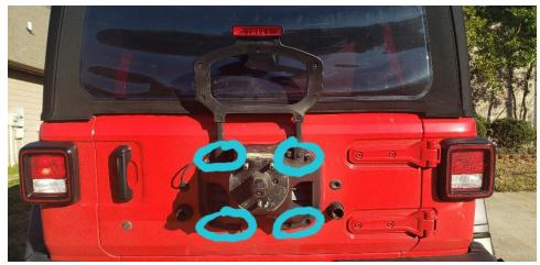
• The next step is to remove the 4 bolts on the hinges, each hinge has 2. To remove these you will need the T-55 torx bit. If you have any issues here it helps to tap the bit in a little to help loosen the factory paint that is around them. Before removing the last bolt I would use tape or something (Pictured) similar and mark where the tailgate lines up with the body so you know that it does not get out of line while installing.
