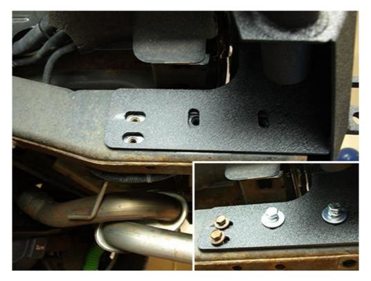
10. Tighten all four (4) middle 18mm M12x110x30 bolts with a Socket Wrench and a 18mm socket along with a 19mm (or standard 3/4) wrench on the lock nut.
