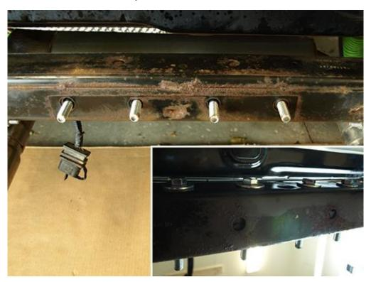
7. Slide the large L bracket into the factory frame on the driver and passenger side as shown below.
