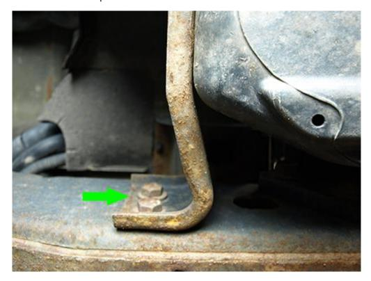
2. Remove the top 16mm bolt that is securing the middle of the factory bumper on the driver and passenger side with a Socket Wrench and a 16mm socket. Then remove the bottom 16mm bolt holding the factory bracket to the frame.
