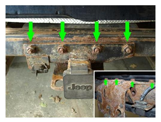
6. Place a M12 flat washer on each of the four (4) M12x110x30 bolts and then slide each bolt through the factory hole from the backside where the factory tow hitch attaches.
