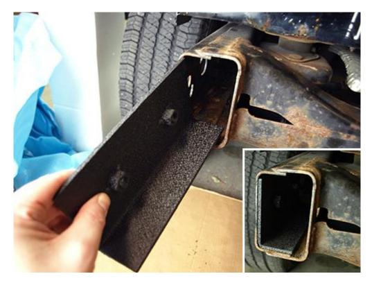
8. With the assistance of another person. Slide the bumper into place making sure the four (4) M12x110x30 bolts slide through the four (4) middle holes of the RedRock 4x4 Crawler Rear Bumper. Place a M12 flat washer, a M12 lock washer and an M12 lock nut on to each bolt. Do Not tighten the lock nuts and bolts yet.
