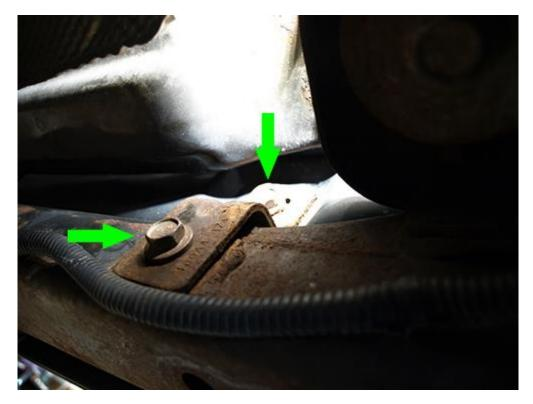
3. Remove the rear factory bumper and place to the side. Note: It is not required to remove the factory spare tire to install the RedRock 4x4 Crawler Rear Bumper.
