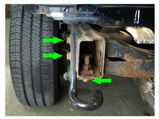
5. **Factory Tow Hitch:** Remove the four (4) 18mm bolts holding the factory tow hitch with a Socket Wrench and a 18mm socket. It's recommended to spray these bolts with a rust penetrating spray if the bolts are extremely rusted.
