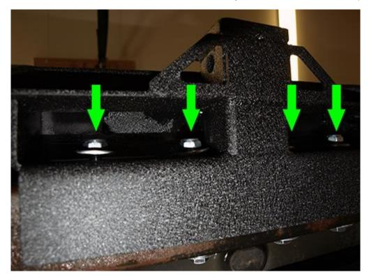
9. Align The outer brackets of the RedRock 4x4 Crawler Rear Bumper to the frame and place the two (2) factory 16mm bolts in the back of the bracket. Then slide a M12 lock washer, a M12 flat washer onto a 18mm M12x40 bolt. Slide this bolt through the outer bracket and secure to the L bracket. Tighten all bolts and repeat the process on the other side.
