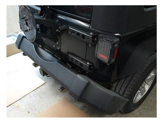
4. Remove the three (3) factory 18mm bolts holding the factory tow hook on the driver side. These bolts may require the use of a breaker bar to break them free. It's recommended to spray these bolts with a rust penetrating spray if the bolts are extremely rusted.
