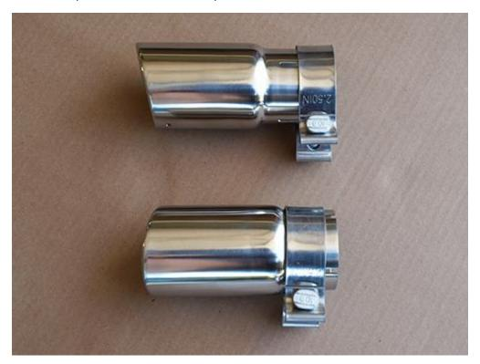
13. Slide one SS Tip onto the driver side of the RedRock 4x4 Exhaust outlet. Align the tip to your personal preference and tighten the nut for the 2.5" band clamp with a socket wrench and 5/8 deep well socket.
