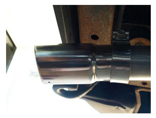
14. Repeat step 13 on the passenger side, and double check the alignment of both SS Tips.
