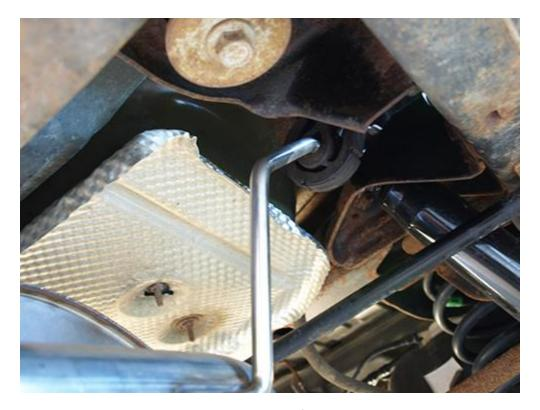
10. Slide the RedRock 4x4 Exhaust metal hanger through the factory rubber hanger to the driver side hanger on the Jeep®. Make sure it slides all the way on to the rubber hanger.
