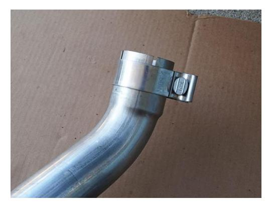
8. Twist the RedRock 4x4 Exhaust until it slides onto the factory exhaust pipe. Do not tighten the nut yet.
