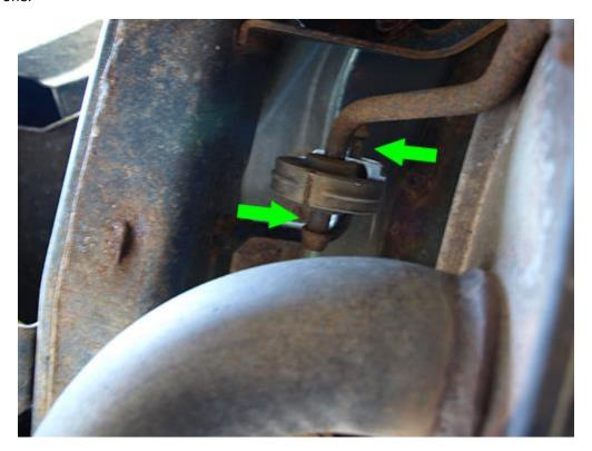
5. Twist and pull the factory muffler until it slides off the exhaust pipe once it's free from hangers on both sides.
