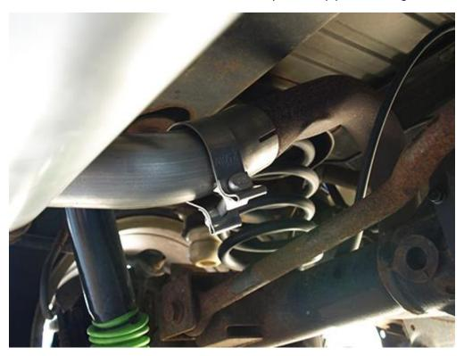
9. Slide the factory rubber hanger that is attached to the RedRock 4x4 Exhaust onto the passenger side metal hanger that is attached to the Jeep®. Make sure it slides all the way onto the metal hanger.
