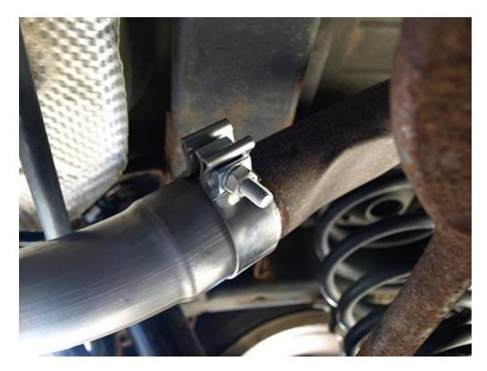
12. Slide a 2.5" band clamp on each end of the SS tips as shown below.
