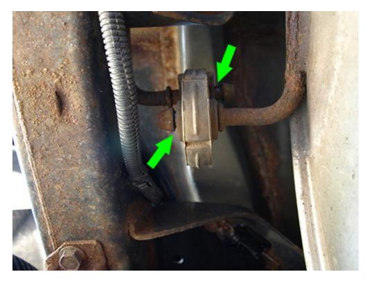
4. Spray a lubricant on both passenger side factory hangers and work the lubrication into the factory rubber hanger. Start to work the top hanger attached to the Jeep® through the rubber hanger using a Large Tongue-and-Grove Pliers or Exhaust/Muffler Hanger Pliers. There is more room to work with the top hanger than the bottom one.
