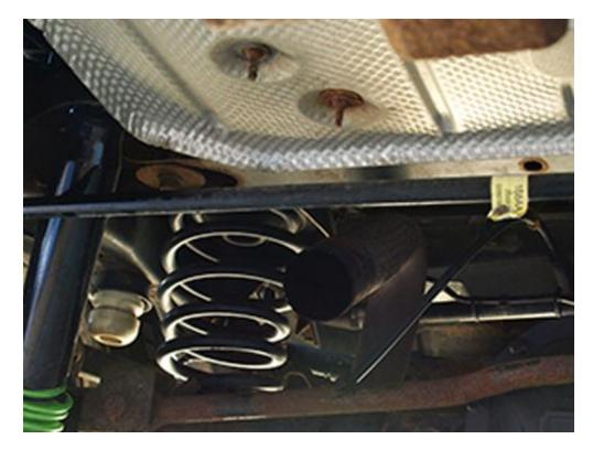
6. Remove the passenger side factory hanger from the factory muffler.
