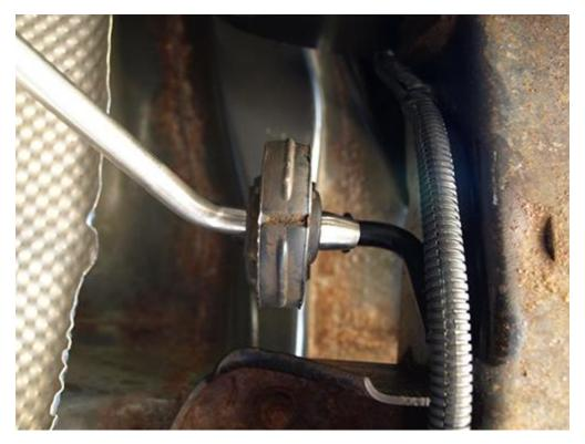
11. Tighten the nut for the 2.5" band clamp with a socket wrench and 5/8 deep well socket.
