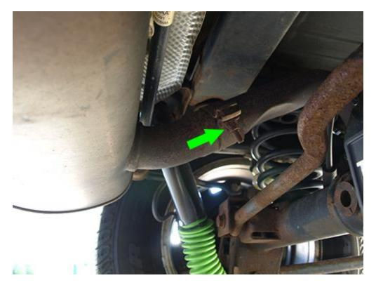
2. Break free the nut that is holding the factory band clap to the exhaust pipe using a socket wrench and 9/16 deep well socket. If the nut is extremely rusted, you may need to use a breaker bar to assist with breaking the nut free. Us a hammer to break the bolt free from the factory clamp.
