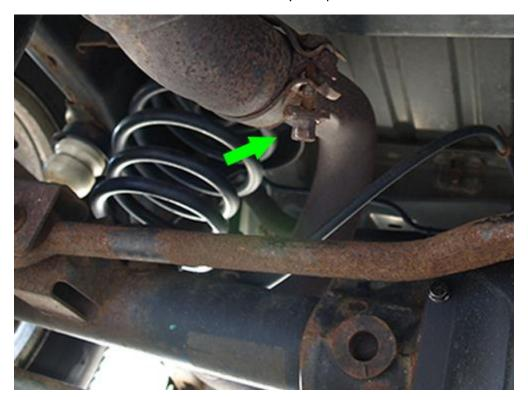
3. Spray a lubricant on both driver side factory hangers and work the lubrication into the factory rubber hanger. Work the bottom metal hanger attached to the muffler through the rubber hanger using a Large Tongue-and-Grove Pliers or Exhaust/Muffler Hanger Pliers.
