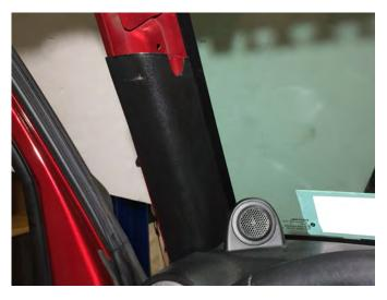
**Step 4\\** Remove the lower trim panel, pull the lower trim away from the body of the vehicle.
