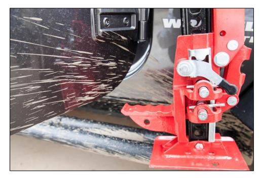
5. Continue to slowly open the door to ensure the Red Rock 4x4 60 in. Extreme Recovery Jack doesn't interfere with the side mirror or any other part of the door when fully open. If there's interference and the jack can't be rotated 180 degrees to remove the interference, try installing the J-Mount on the upper windshield hinge mounts.
