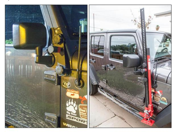
2. Remove BOLT lock cylinder and J-Mount plastic knobs. Place jack into position on BOLT post for a test fit.
