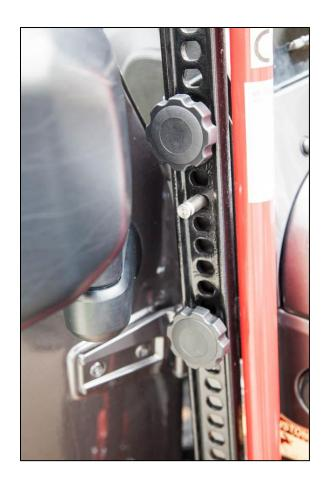
6. Reinstall the BOLT lock cylinder to fully secure the jack to the Jeep.
