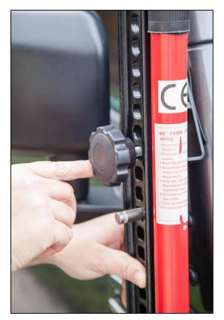
4. Slowly open the Jeep door to ensure the foot of the Red Rock 4x4 60 in. Extreme Recovery Jack doesn't interfere with the bottom of the door. If there's interference and the jack can't be raised or lowered, rotate the jack 180 degrees so the foot faces the fender flare.
