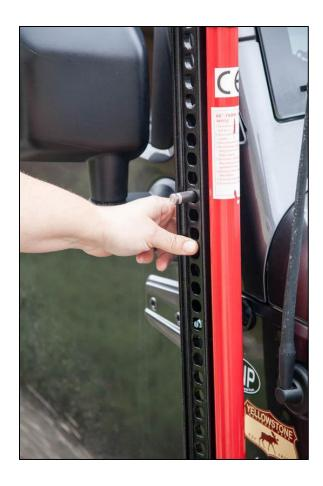
3. Reinstall the plastic retaining knobs to secure the Jack while continuing the test fit.
