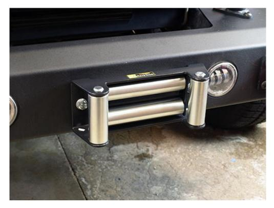
11. Place the winch on your bumper or winch plate. Before securing the winch cut the large zip tie holding the steel cable to the Tie Bar/Rail. Move the Clutch handle on the winch to Free Spool. The steel cable will loosen. Slide the cable through the Roller Fairlead and set the clutch back to Engaged.
