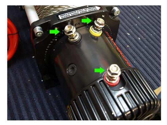
7. Place the black cable with the black boot from the Solenoid on to the color-coded black post of the motor end. Tighten down with a 13mm open ended wrench. Then slide the wire boot over the post.
