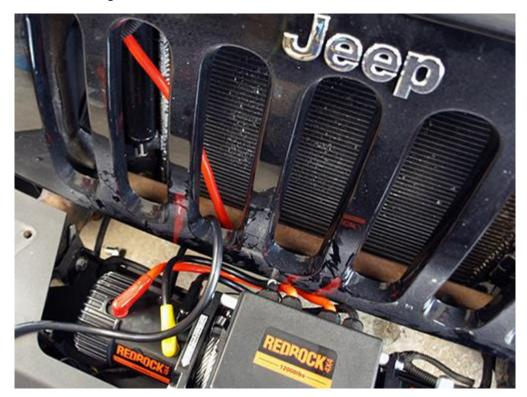
16. Run the red power wire to the positive battery terminal and the black ground wire to the negative battery terminal.
