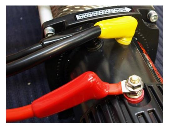
9. Place the winch on its side. Remove the nut from the bottom post and slide the small black cable coming from the Solenoid to this post. Now place the Long Black Ground Wire onto the same post. Screw the nut back on and tighten down using a 16mm open ended wrench. Then slide the wire boot over the post.
