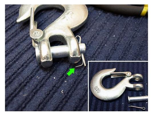
13. Slide steel cable loop between the Safety Hook opening and then slide the large pin back through the hook. Slide the Cotter Pin through the hole of the large pin and bend the longer end using a needle nose pliers to the side as shown below.
