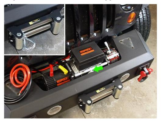
12. Remove the Cotter Pin from the Safety Hook using a needle nose pliers and remove the large pin from the hook.
