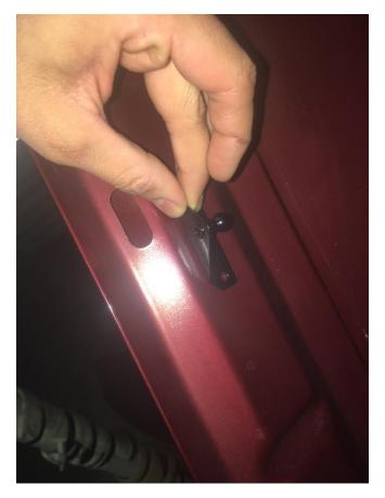
6. Place a mark in the center of the lower hole and upper hole using the marker. (Make sure the bracket is straight and flat against the hood's frame
