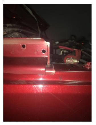
13. Place one washer onto the ball-stud and insert it into the hole facing inward. Put lock nut onto the shaft. Use  $\chi''$  socket to tighten the lock nut.
