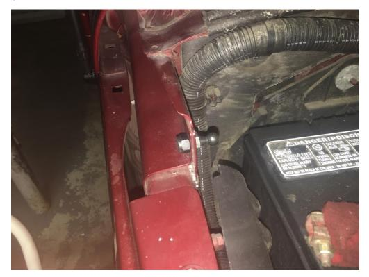
15. Snap gas springs onto the ball studs.
