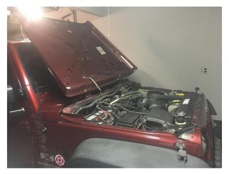
3. Measure from the lower edge of the hood 21" up and place a mark.
