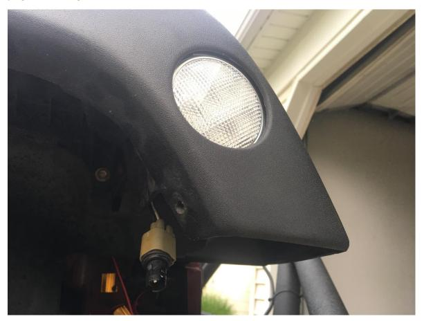
9. Plug the light assembly back in making sure it is plugged in, in the correct direction and working. Re-install the things taken off the fender in step 6.
