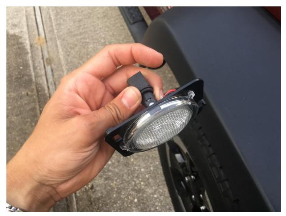
5. Plug the light into the harness and see if it is working correctly.
