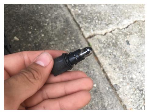
3. Remove the light from the plastic piece it is in by pulling it out.
