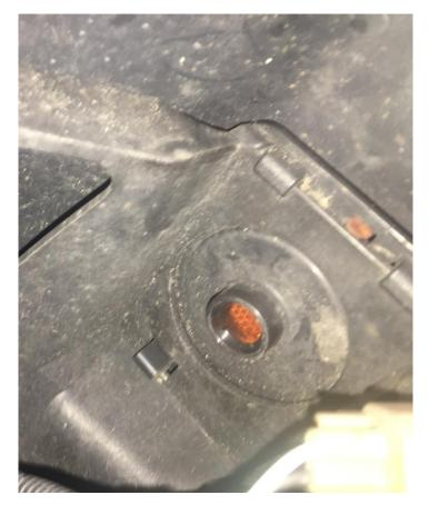
8. Unplug the Recon light and insert it into the fender.
