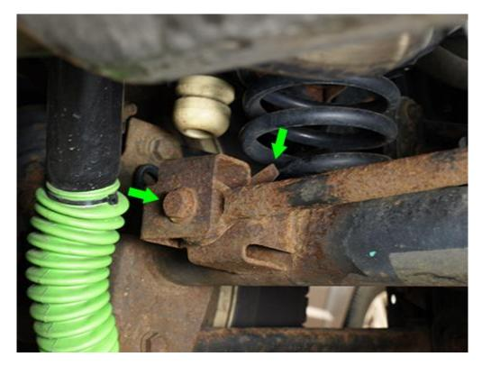
2. Remove the factory rear track bar bolt attached to the body bracket with a Socket Wrench with a 21mm socket and a 6" extension on the bolt head. Place a Open Ended 21mm wrench on the nut. You may need to use a breaker bar to break this bolt free. Slide the factory rear tracker bar down once it's free.
