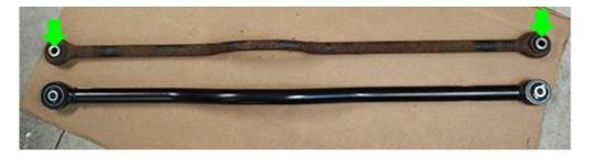
4. Place the ReadyLIFT Rear Adjustable Track Bar into the body bracket and slide the factory 21mm bolt through to the other side and screw on the 21mm nut. Loosely tighten the nut.
