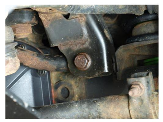
3. Lay the factory track bar above the ReadyLIFT Front Adjustable Track Bar and measure from the passenger side metal bushing to the driver side metal bushing. Transfer this measurement to the ReadyLIFT Front Adjustable Track Bar, and loosely tighten the jam nut the orange arrow is pointing to below.
