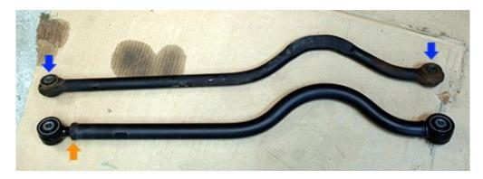
4. Place the ReadyLIFT Front Adjustable Track Bar into the body bracket and slide the factory 21mm bolt through to the other side and screw on the 21mm nut. Do not tighten yet.
