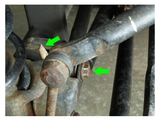
2. Remove the driver side factory front track bar bolt attached to the body bracket with a Socket Wrench and a 21mm socket and an Open Ended 21mm wrench on the nut. May need to use a breaker bar to break this bolt/nut free.
