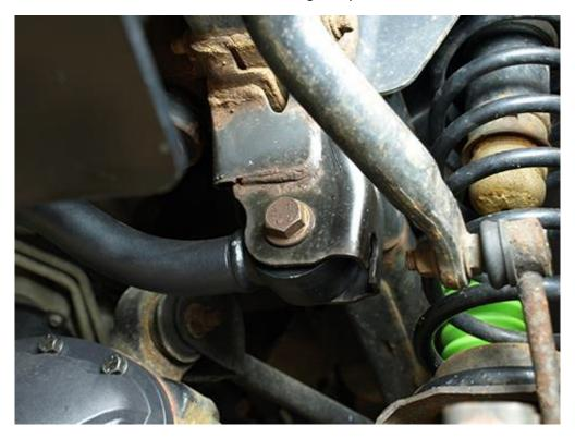
5. Place the passenger side of the track bar into the axle bracket and slide the 21mm factory bolt through and screw into the capture nut. With the Jeep® on the ground under its own weight. Torque the body bolt and the axle bolt to 125-foot pounds. Using a Tongue-and-Grove Pliers. Tighten the jam nut as tight as you can.
