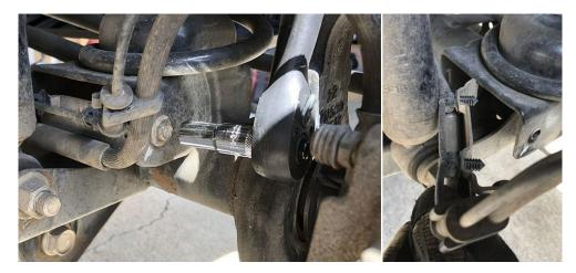
3. Remove the bottom sway bar link bolt where it connects to the axle using a 18mm wrench
