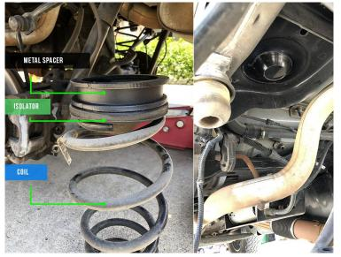
14. Jack up the axle and proceed to reinstall the components in reverse order. Install the lower shock bolt and torque to 56 ft/lbs, sway bar link (torque to 75 ft/lbs) and ABS wire bracket (Hand tight). Repeat the steps on the passenger side of the vehicle. Push the plastic rivets back into their places. Once both sides are completed, reinstall the wheels and torque the lugnuts to 110 ft/lbs.
