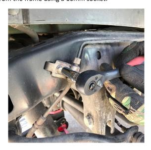
10. Remove the lower swaybar link using a 18mm wrench or two Crescent wrenches.
