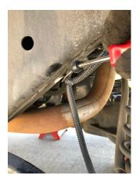
13. Lower the axle down and remove the coil and isolator. Place the new spacer on and facing downward. Next comes the isolator, then finally the coil. Place them back in and ensure that the spacer is properly seated at the top. Repeat on opposite side.
