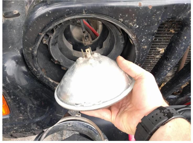
2. Align your new LED light with the surround and after passing harness through opening, raise into place and secure with retaining ring. For correct orientation, accent bar should be horizontal and letters DOT should be
