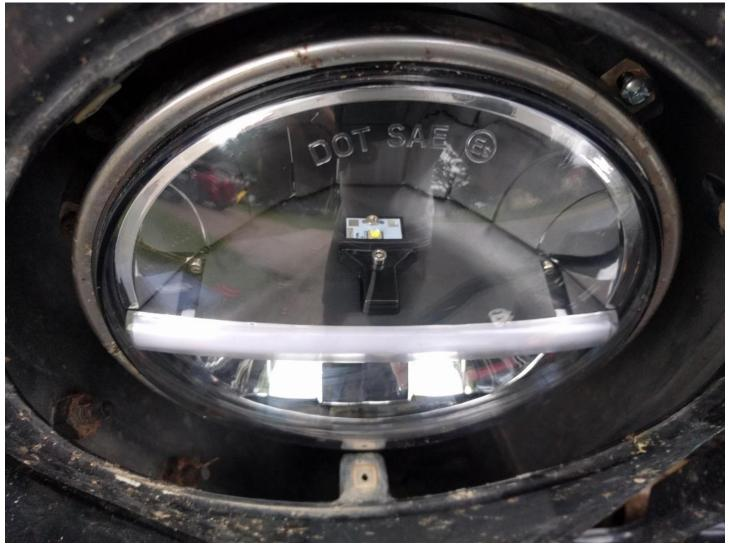
3. From inside engine bay, connect Jeep-side harness to light harness. If installing on a JK, LED Canbus and harness adapter must be used, on a TJ they are not necessary. Next identify two additional wires on light harness. Red is Running Light (White Accent Bar), Green is Turn Signal (Amber Accent Bar). These wires will tie-in with factory running/indicator lights using your butt connectors, splice taps, and bulk wire.
