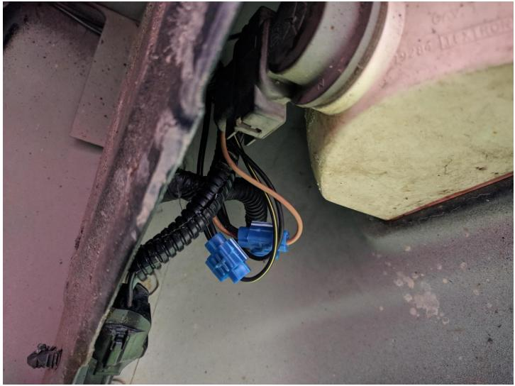
5. If desired, install wire loom over new wire runs for additional protection. Verify functionality of all light functions and then reinstall outer bezels.
